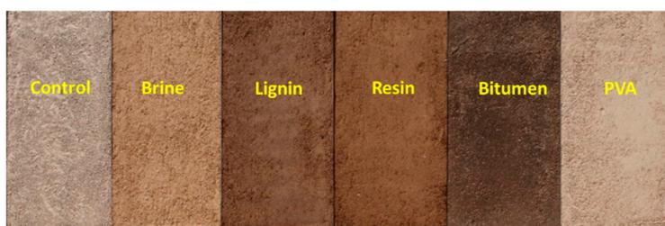
**Figure 2.** The soil samples in trays after the application of the dust control product used for the laboratory wind tunnel experiment. The size of each tray is  $0.5 \times 1.0$  m with height of 0.02 m. each soil sample was prepared in three replicas.
