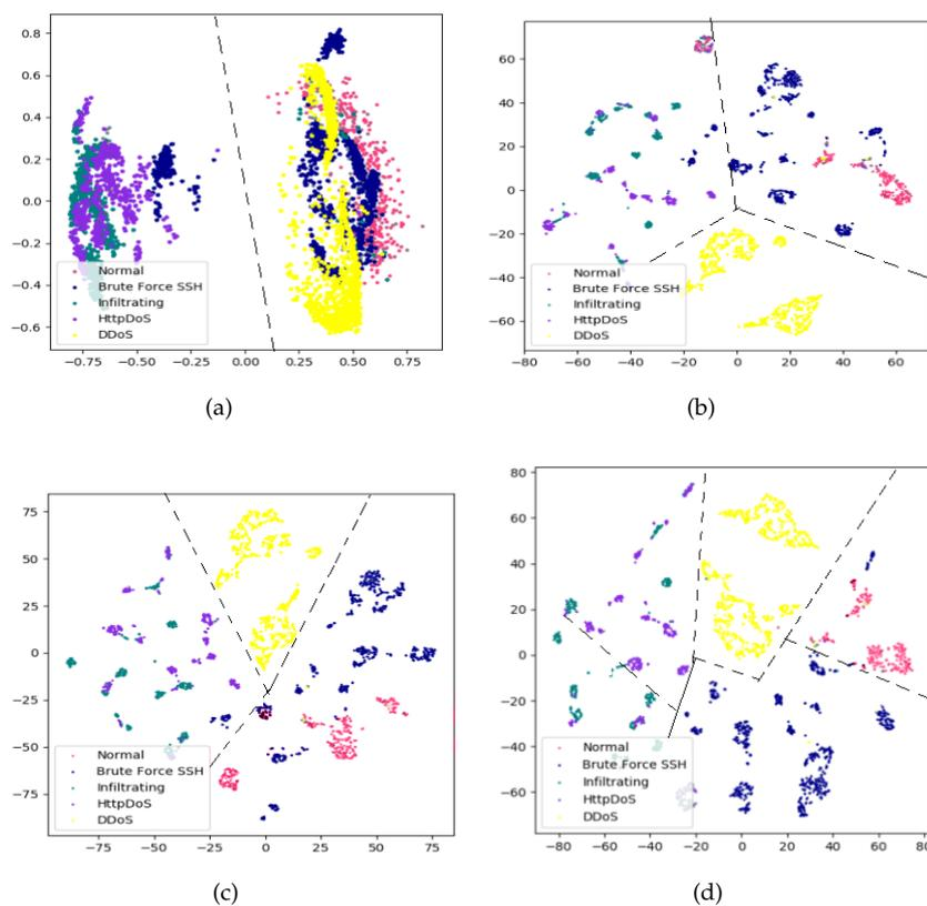
**Figure 7.** Visualization of unsupervised intrusion detection algorithms. (a) PCA algorithm. (b) Deep Auto-encoder algorithm. (c) Proposed node2vec-AE algorithm. (d) Proposed packet2vec-AE algorithm.
