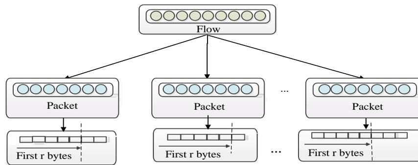
**Figure 3.** Splitting the originally traffic into packets. The original traffic is split into packets to be truncated into fixed length.
