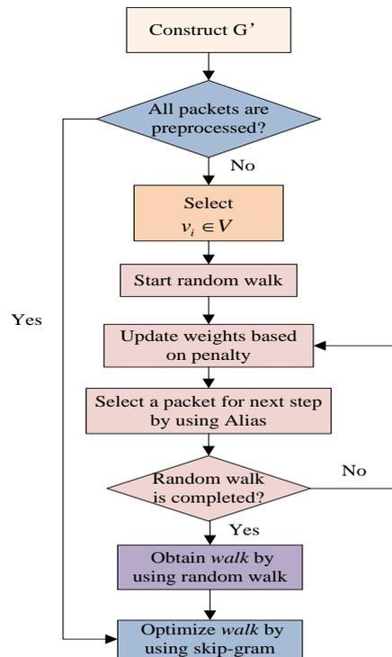
Figure 4. Algorithmic flowchart of packet2vec learner based on graph representation with penalty.
