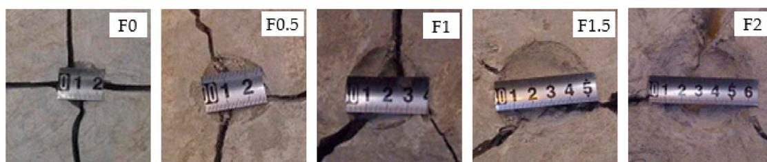
Figure 4. Impact craters of PVA-FRCM disc specimens.
