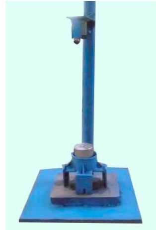
(b) Self-improved equipment for drop-weight test
