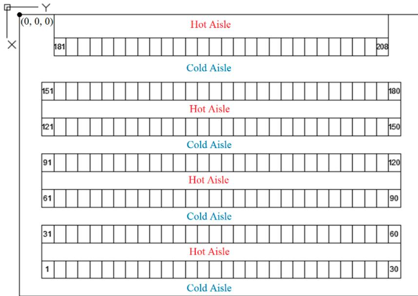
Figure 3. The representation of upper plan view of the data center room.
