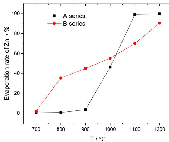
**Figure 3.** The effect of the reducing agent on the reduction and evaporation of zinc.
