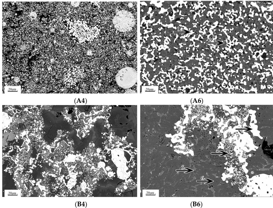
**Figure 5.** The microstructure of the sample after being reduced at 1000 °C and 1200 °C (A4 and A6 were reduced by carbon at 1000 °C and 1200 °C, respectively. B4 and B6 were reduced by ferrosilicon at 1000 °C and 1200 °C, respectively).
