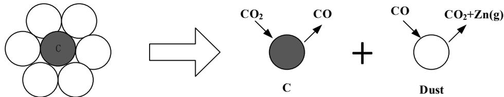
**Figure 7.** Schematic diagram of the reaction of EAFD containing zinc reduced by carbon.
