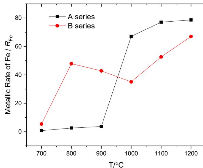
**Figure 4.** The effect of the reducing agent on the percentage metallization of iron.
