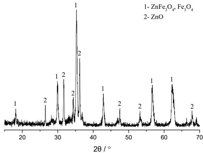
Figure 1. XRD diffraction pattern of EAFD.
