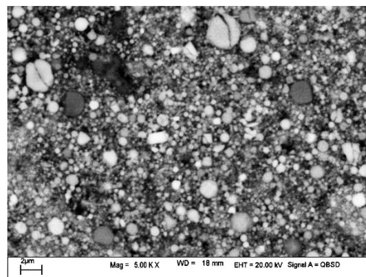
Figure 2. The microstructure of EAFD.
