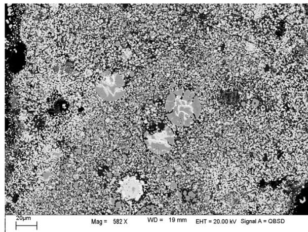
**Figure 9.** The microstructure of samples in B2 reduced at 800 °C.
