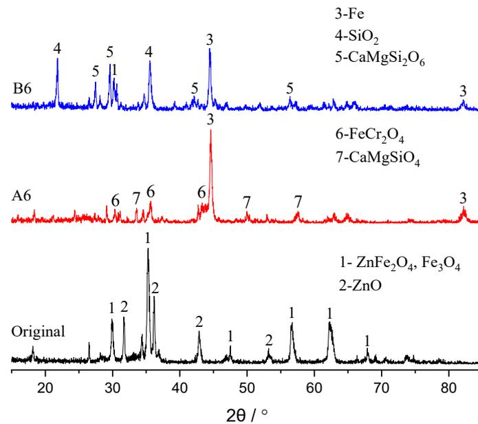
Figure 6. The mineral components of the samples obtained at 1200 °C.
