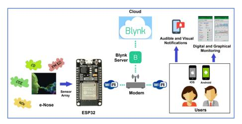
Figure 1. The proposed e-nose system architecture.
