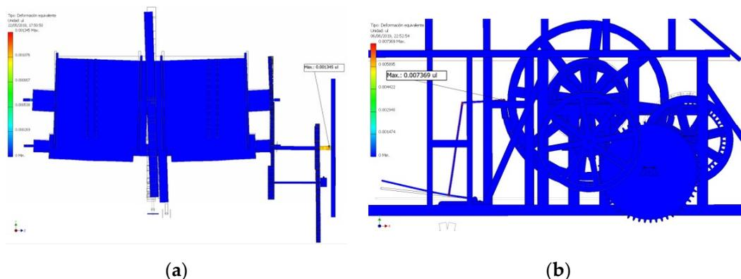
Figure 24. Location of the highest deformation: (a) blockage situation and (b) braking situation.
