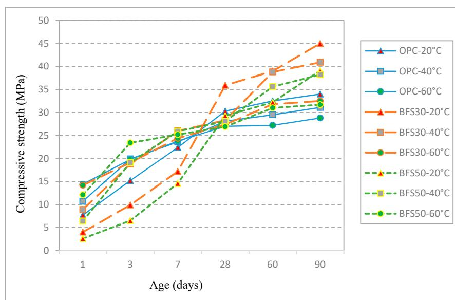
**Figure 6.** Compressive strength (MPa) at various water curing temperatures and ages for OPC and slag blended cement mortars (BFS30 and BFS50).**Table 3.** COE records with 20–60 °C increase in water curing temperature at ages up to 90 days for OPC and slag blended cement mortars.
