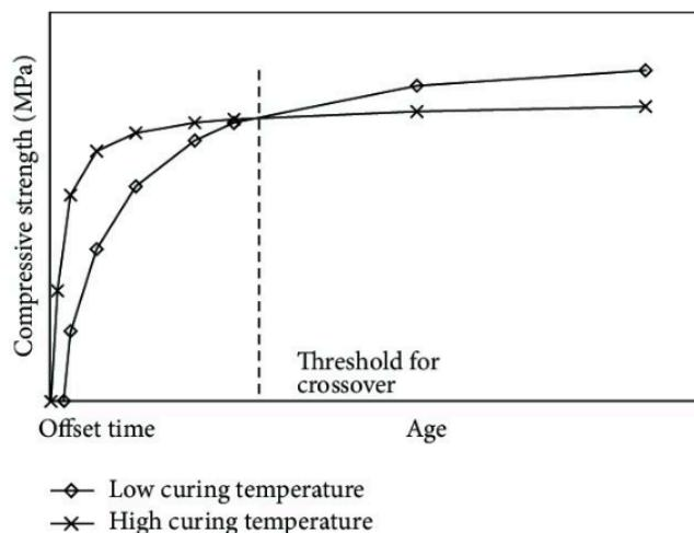
**Figure 2.** COE during strength development of concrete due to different initial curing temperatures.
