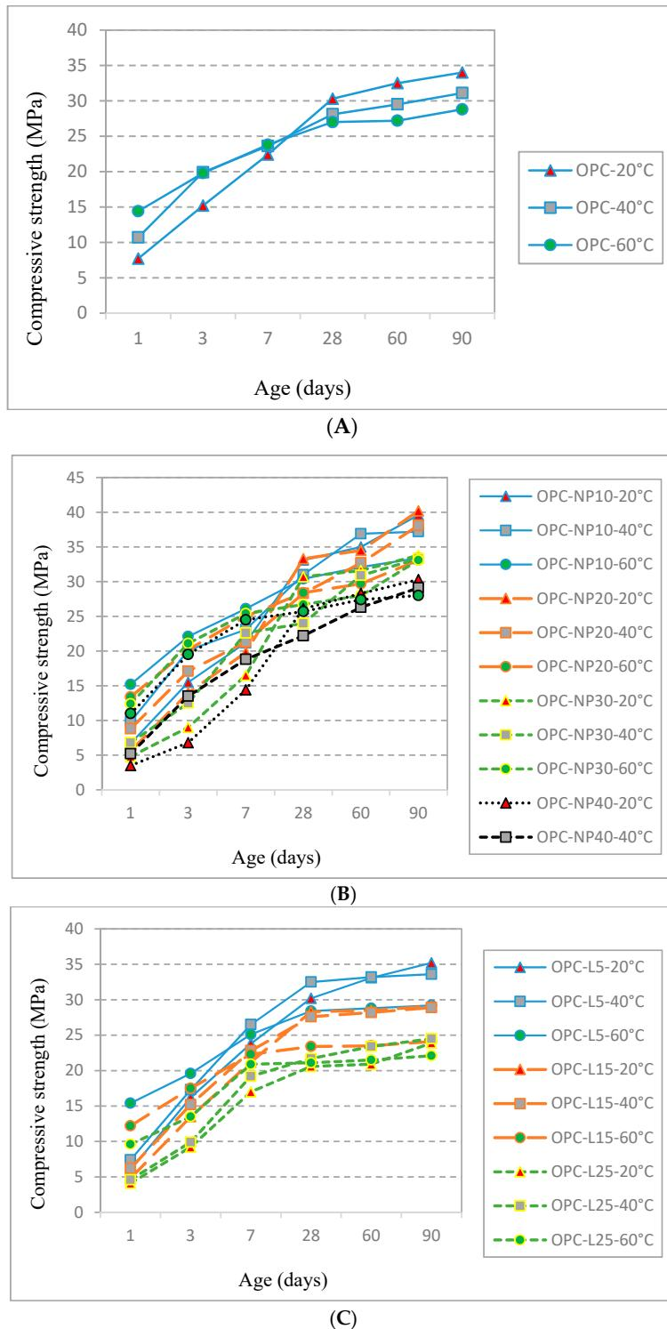
**Figure 8.** Compressive strength (MPa) at various water curing temperatures and ages for (A) OPC; (B) natural pozzolan blended cement; (C) limestone powder blended cement mortars.
