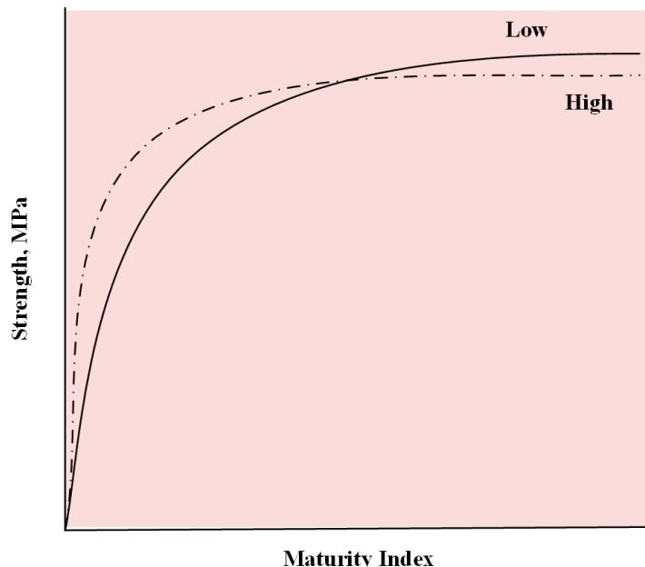
**Figure 1.** Crossover effect (COE) with maturity and strength at low and high temperatures.
