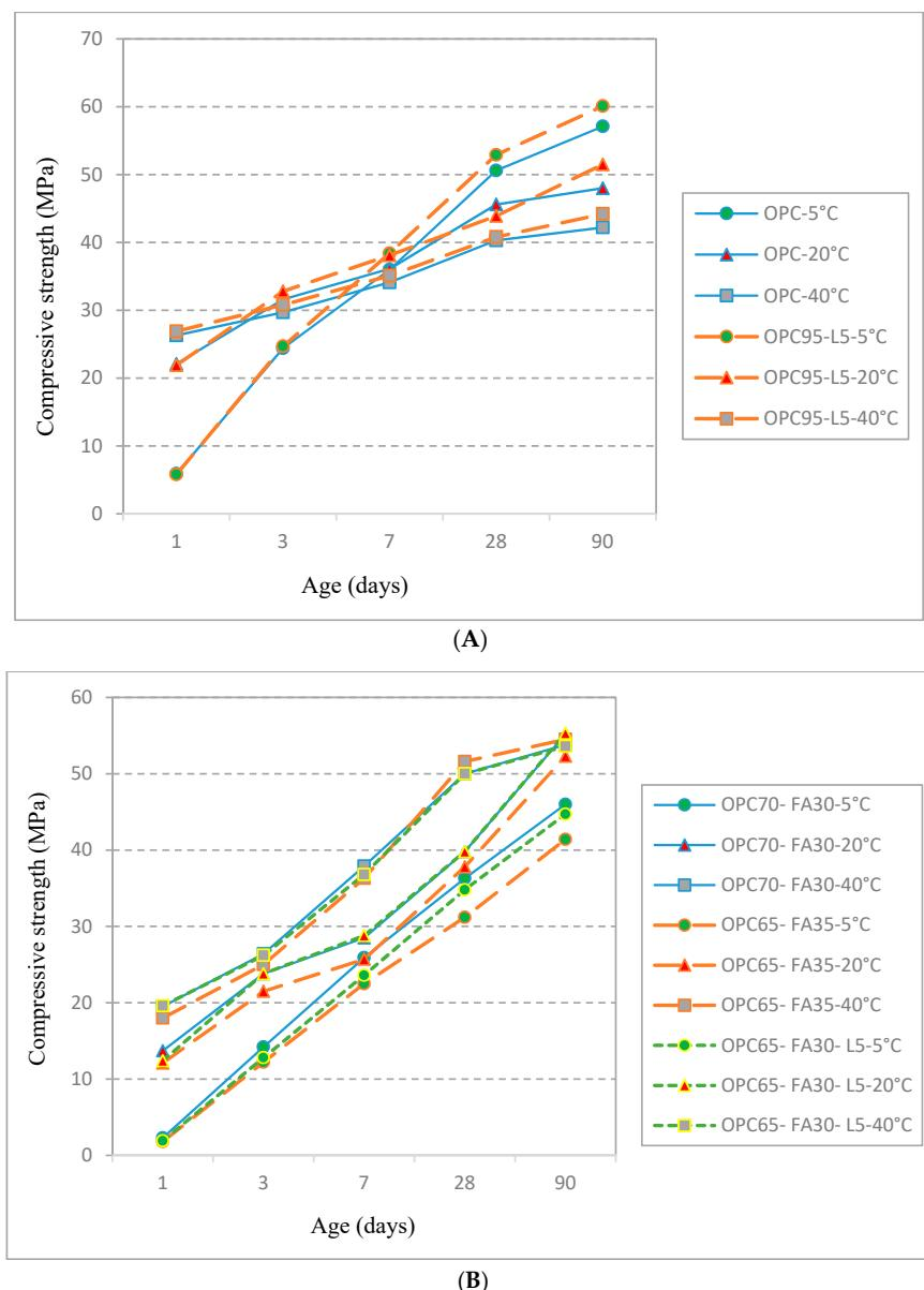
**Figure 7.** Compressive strengths (MPa) of (A) OPC and OPC95-L5; (B) OPC70-FA30, OPC65-FA35 and OPC65-FA30-L5 for water curing temperatures of 5 °C, 20 °C and 40 °C.
