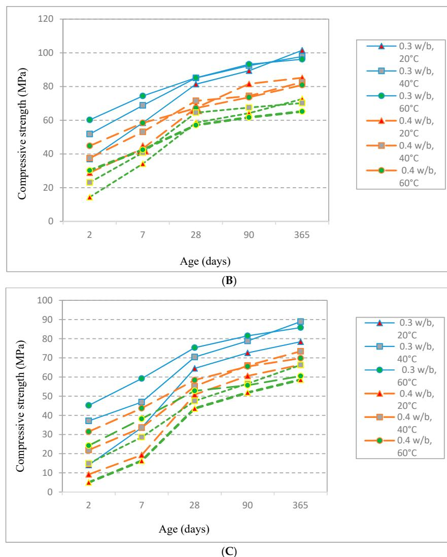
**Figure 5.** Compressive strength (MPa) at various water curing temperatures and ages for (A) OPC; (B) BFS40; (C) BFS80 pastes.
