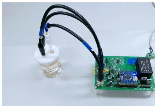
**Figure 4.** The designed voltammetry electronic tongue hardware system.
