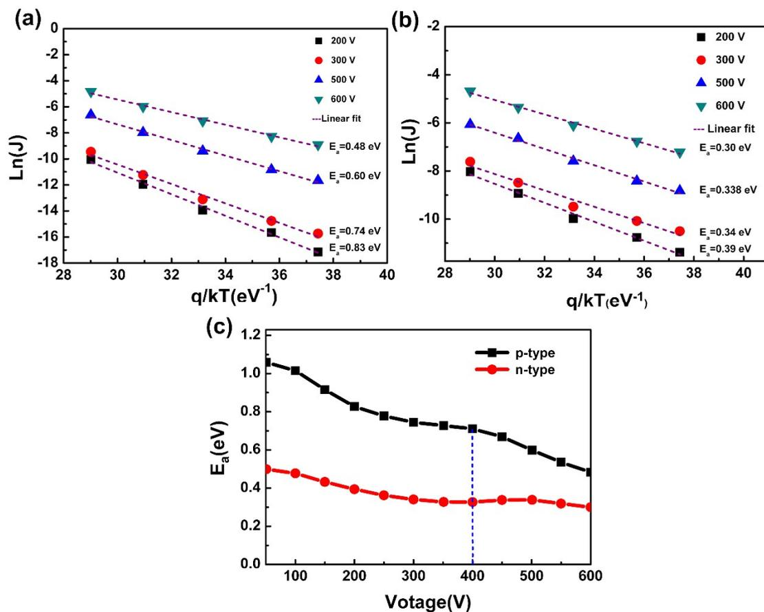
**Figure 3.**  $E_a$  extracted from  $\ln J-1/T$  at different biases of p-type (a), and n-type (b) samples, (c)  $E_a-V(T)$  plots of p-type and n-type samples.
