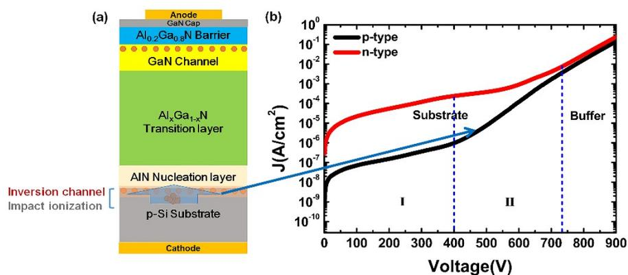
**Figure 1.** Growth structure with p-Si (111) substrate (a). Measured vertical leakage current of grown structures on p-Si and n-Si (111) substrate (b).
