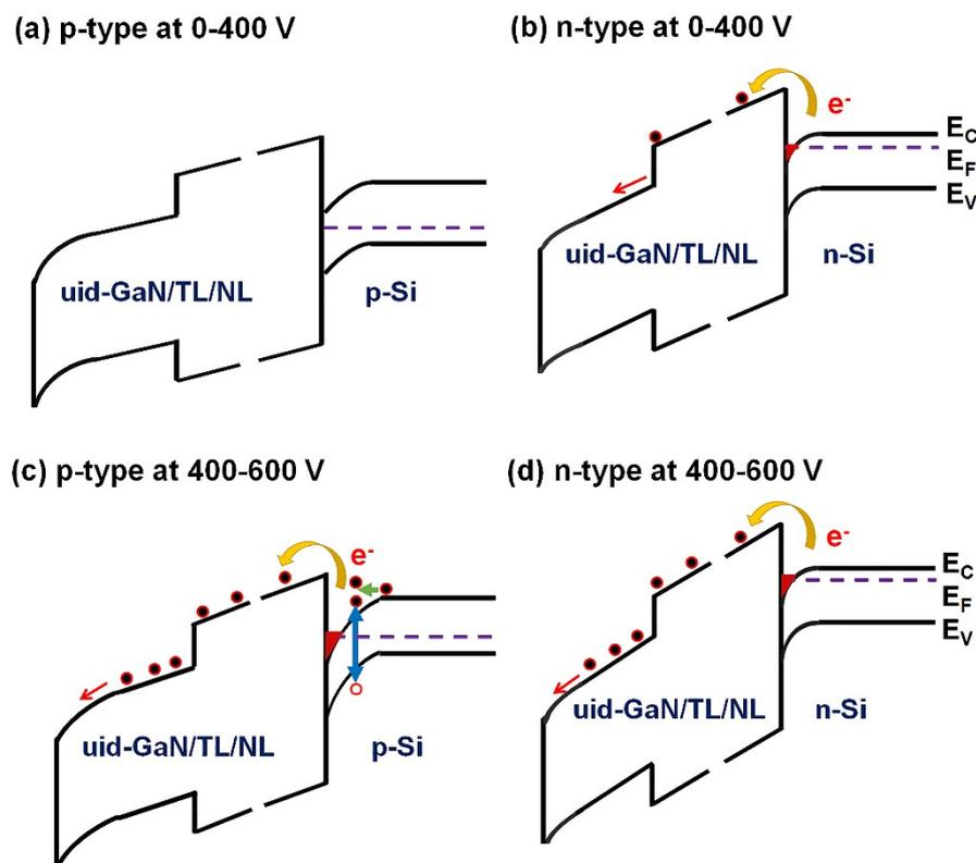
**Figure 4.** Band diagrams of the GaN-on-Si structure when the top surface is forward biased. (a) p-type, (b) n-type for 0–400 V and (c) p-type, (d) n-type for 400–600 V.
