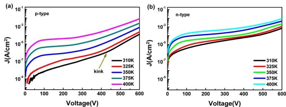
**Figure 2.** Temperature-dependent current-voltage (I-V) characteristics of p-type (a), n-type samples (b).
