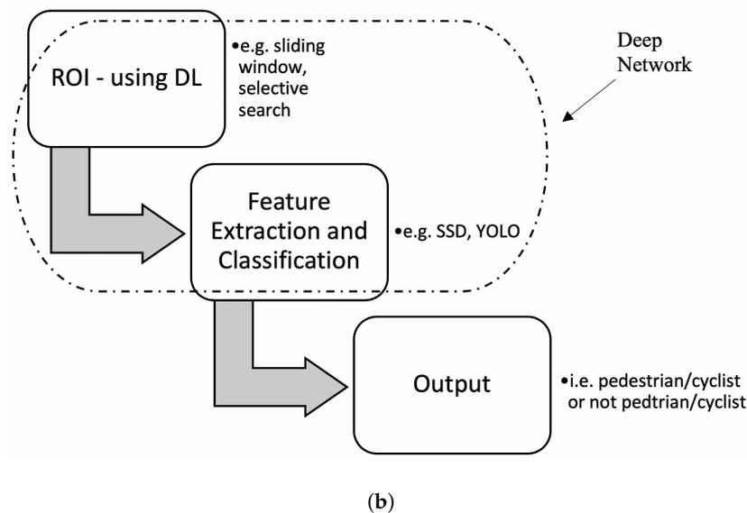
**Figure 6.** Architectures for CNNs for feature extraction and classification based on traditional methods for (a) Non-Region Proposal-based Detectors and DL methods for (b) Region Proposal-based Detectors.
