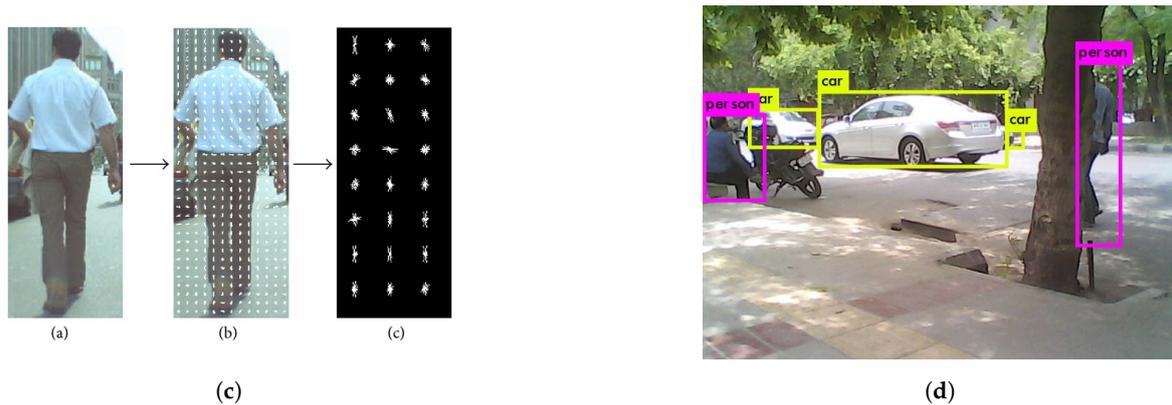
**Figure 2.** Basic Detection System Structure: (a) the sensor system captures data in the form of an image (b) region proposal techniques are applied, (c) features are extracted from the proposed regions and (d) finally the features are fed into a classifier. (a) Sensor System [55]. (b) Region Proposal [56]. (c) Feature Extraction [57]. (d) Classification [58].
