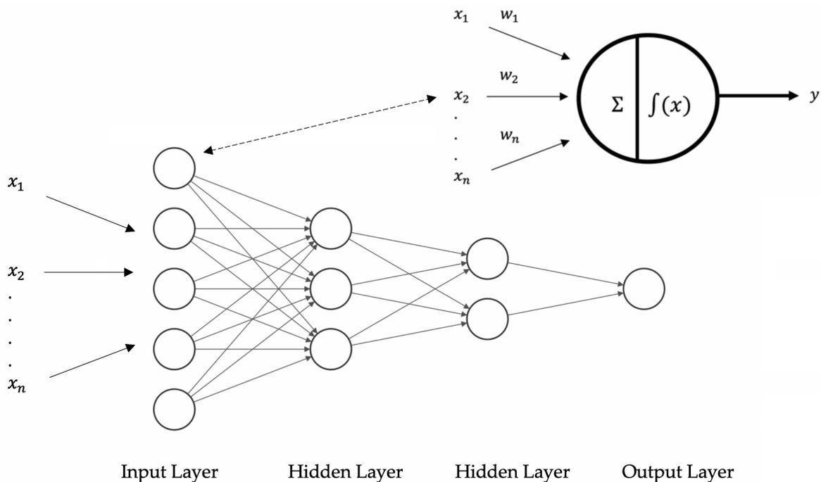
Figure 4. The architecture of a multilayer perceptron.
