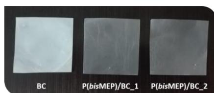
**Figure 1.** Visual aspect of a dry pure BC (bacterial cellulose) membrane, and P(*bis*MEP)/BC\_1 and P(*bis*MEP)/BC\_2 nanocomposites.
