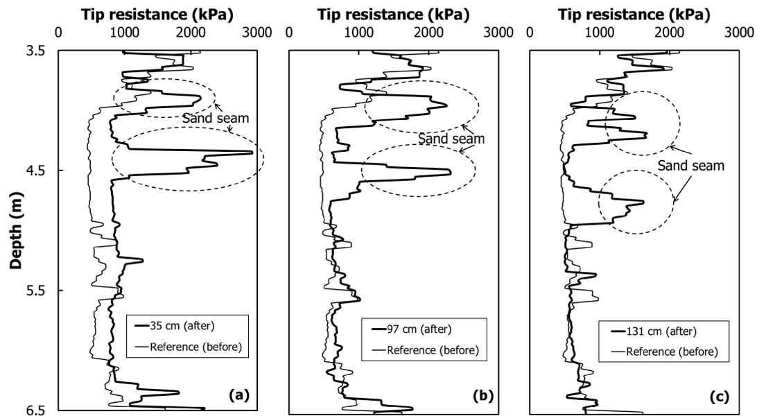
Figure 11. The variation of the tip resistance due to ground heating using an electric heat pipe (Case 4), (a) a point 35 cm in the horizontal direction; (b) 97 cm; (c) 131 cm.
