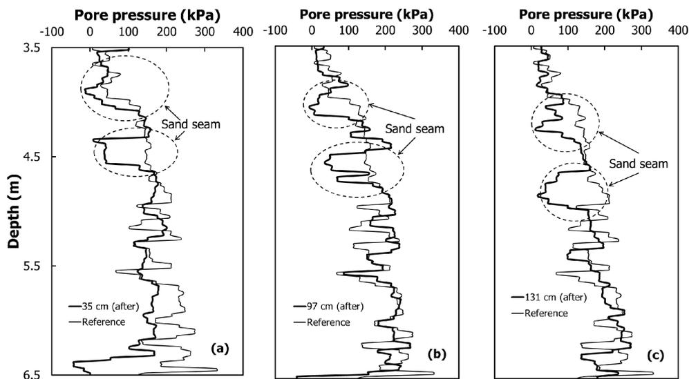
**Figure 15.** The variation of the pore pressure according to the horizontal distance from the electric heat pipe (Case 4), (a) a point 35 cm in the horizontal direction; (b) 97 cm; (c) 131 cm.
