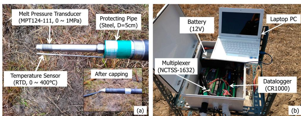
**Figure 5.** The installation process of the sensors and the measurement systems. (a) Installed sensors; (b) measurement system.
