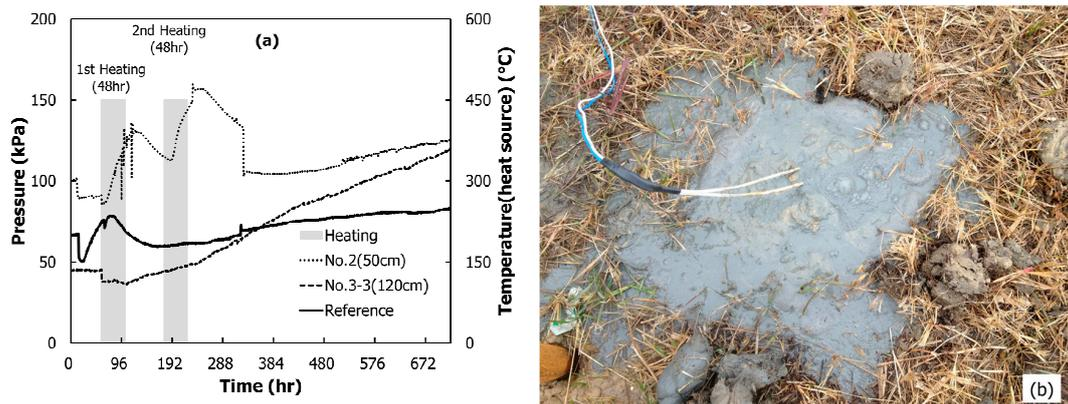
**Figure 9.** The variation of the vapor pressure by ground heating using an electric heat pipe. (a) The variation of the vapor pressure; (b) the bubbles on the ground surface.
