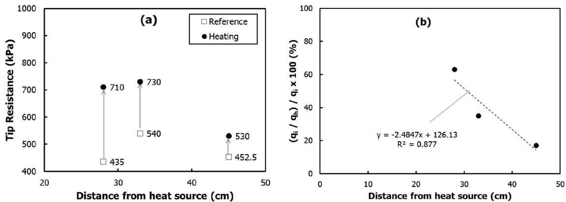
**Figure 14.** The variation of the tip resistance according to the distance from the surface of the electric heat pipe (Cases 5, 6 and 8), (a) the comparison of the variation in tip resistance before and after heating; (b) the comparison of the increased rate of tip resistance after heating.
