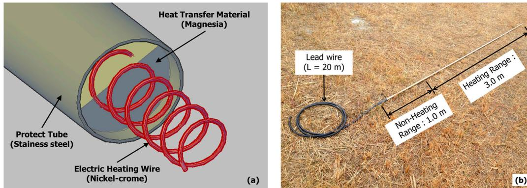
Figure 3. The electric heat pipe in the field test. (a) Section view; (b) Overall view.
