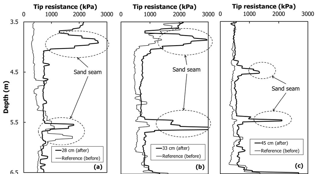
Figure 12. The variation of the tip resistance due to ground heating using an electric heat pipe (Cases 5, 6, and 8), (a) a point 28 cm in the horizontal direction; (b) 33 cm; (c) 45 cm.
