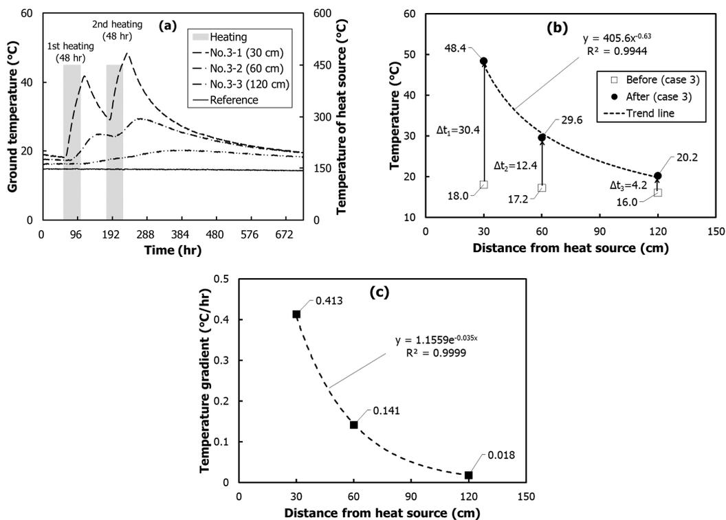
**Figure 8.** The temperature variation by ground heating using an electric heat pipe. (a) The temperature variation of all the sensors; (b) the variation of the temperature curve; (c) the temperature gradient according to the distance from the surface of the electric heat pipe.
