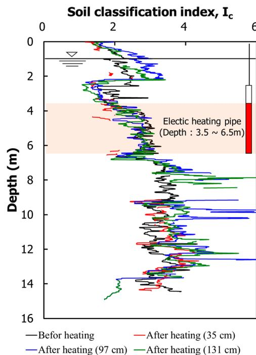
**Figure 10.** The Soil Classification Index obtained by the CPT tests data (before and after ground heating).
