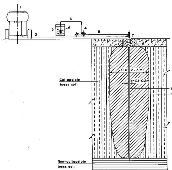
**Figure 1.** The conceptual diagram of the ground heating method using fossil fuel proposed by Litvinov [22].
