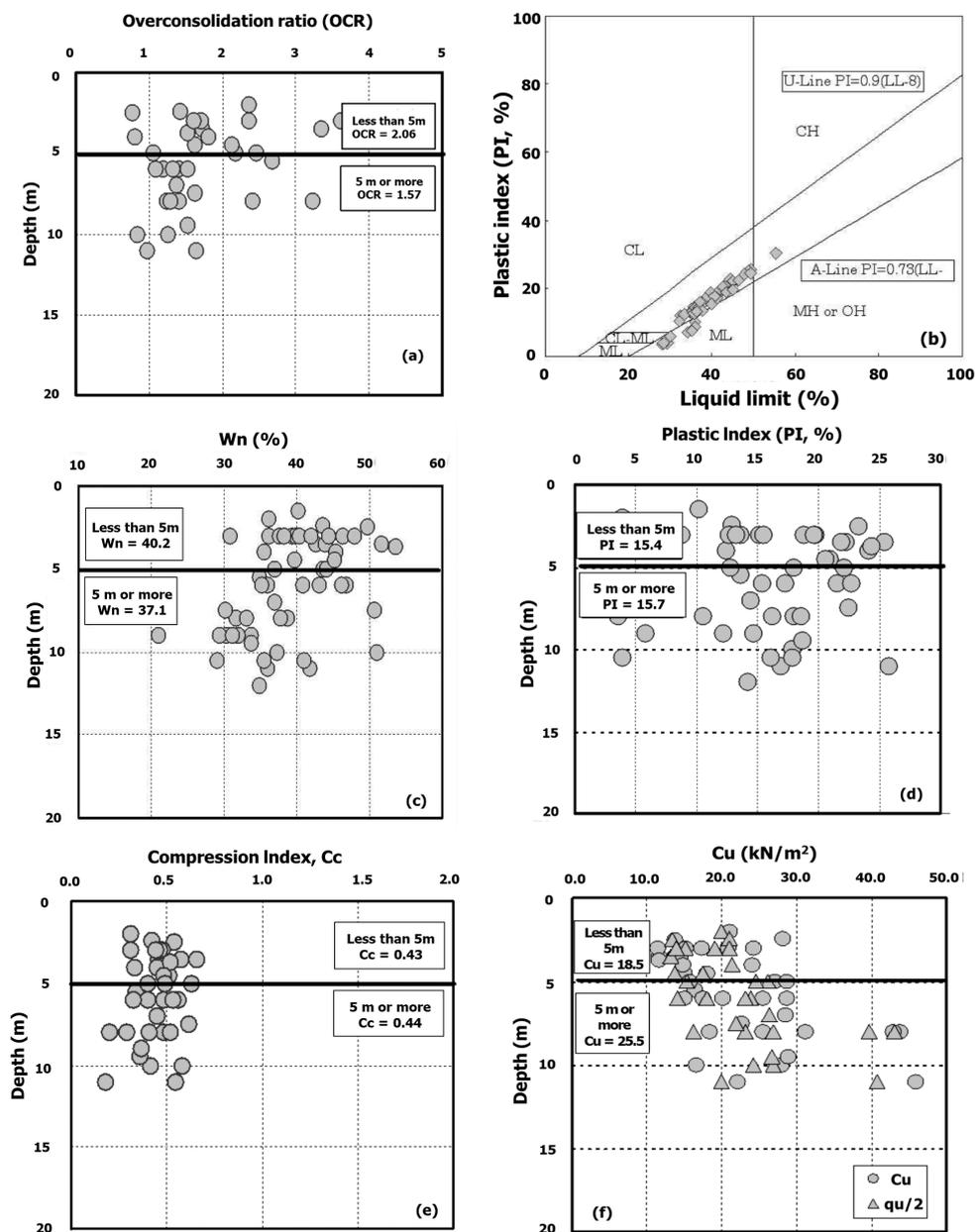
**Figure 4.** The geotechnical and physical properties of clay. (a) over-consolidation ratio; (b) plasticity chart; (c) natural water content; (d) plasticity index; (e) compression index; (f) undrained shear strength.
