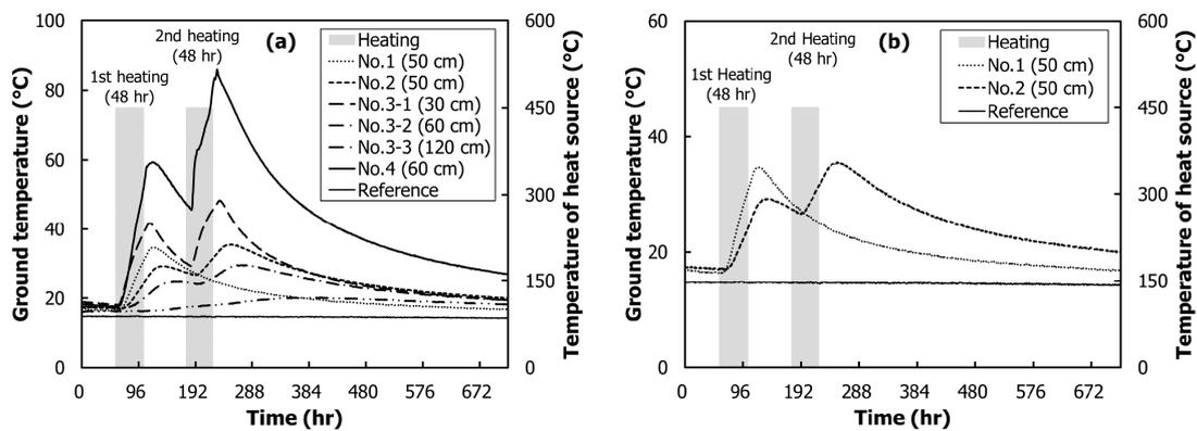
Figure 7. The variation of the ground temperature due to ground heating. (a) Overall sensor; (b) comparison of the temperature variation due to the installation of the steam discharge hole.
