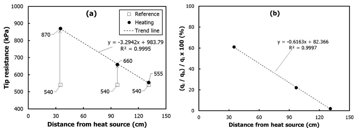
**Figure 13.** The variation of the tip resistance according to the distance from the surface of the electric heat pipe (Case 4); (a) the comparison of the variation in the tip resistance before and after heating; (b) the comparison of the increased rate of tip resistance after heating.
