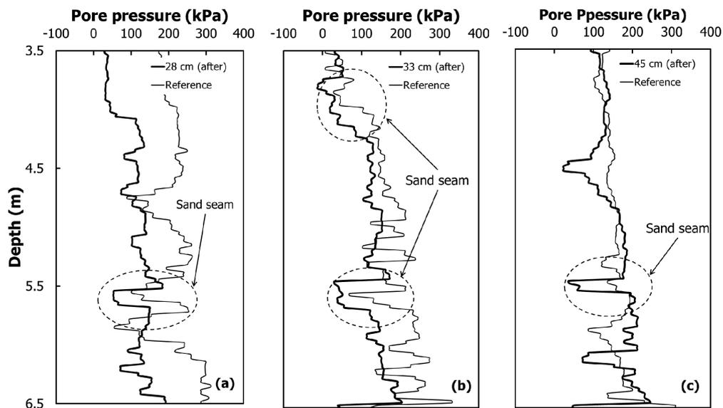
**Figure 16.** The variation of the pore pressure according to the horizontal distance from the electric heat pipe (Cases 5, 6 and 8), (a) a point 28 cm in the horizontal direction; (b) 33 cm; (c) 45 cm.
