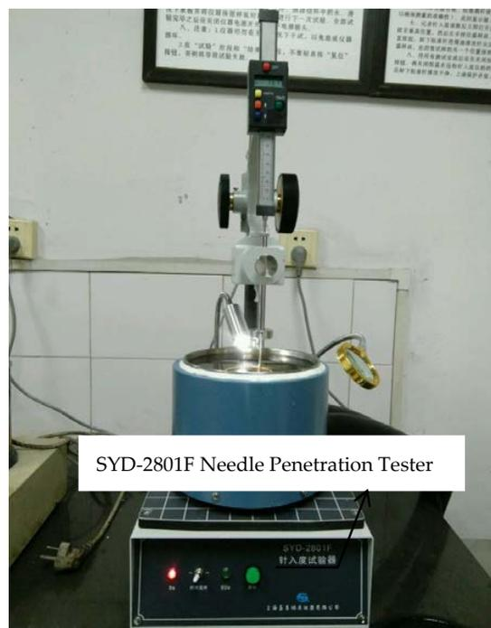
Figure 6. The Needle Penetration Tester.
