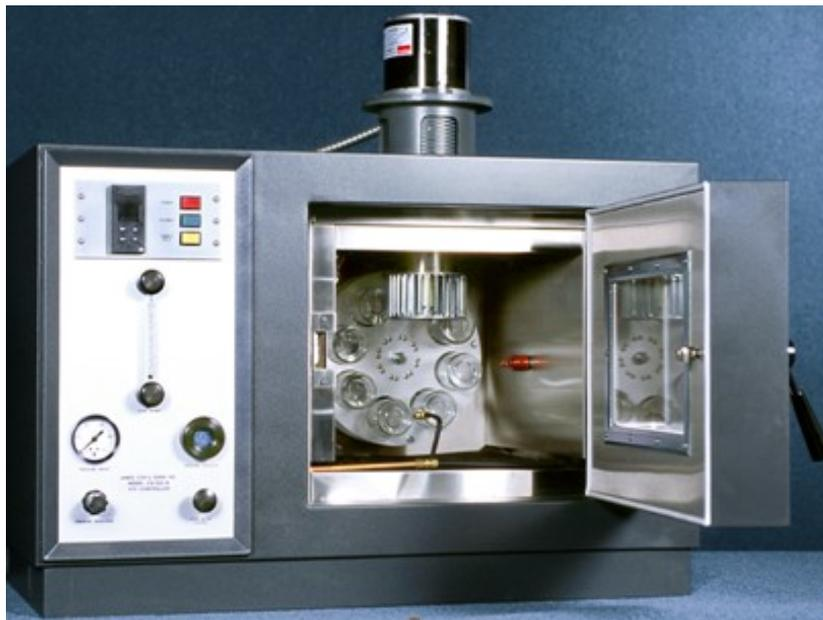
Figure 5. The Rolling Thin Film Oven.
