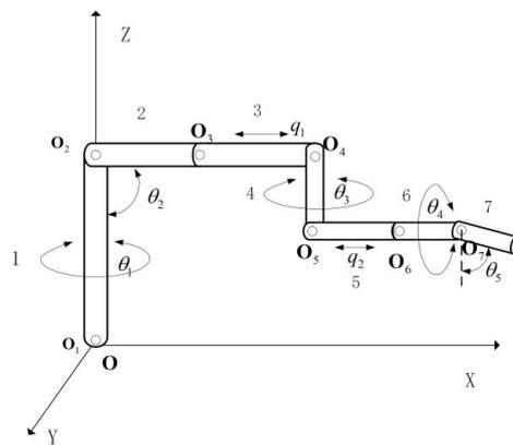
Figure 4. The 7-DOF manipulator coordinate diagram.
