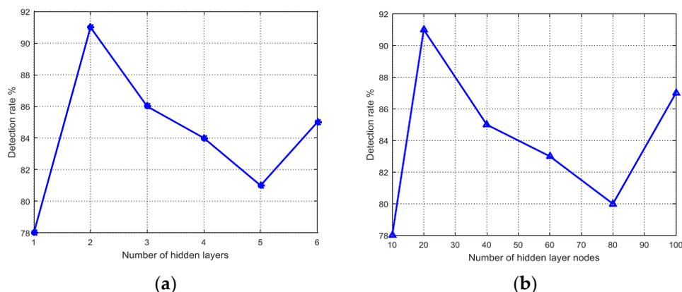
**Figure 3.** (a) The correct detection rate changes with the number of hidden layers (20 nodes); (b) The correct detection rate varies with the number of hidden layer nodes (2 hidden layers nodes).
