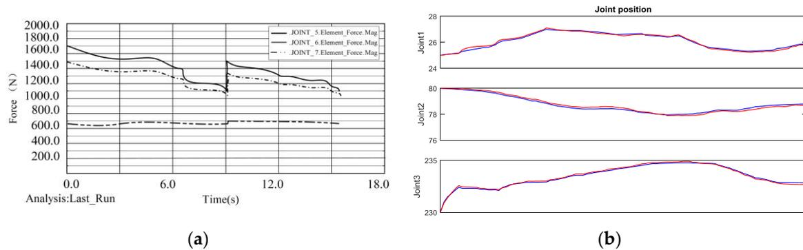
Figure 6. (a) The forces of three joints in Adams; (b) Trajectory following.
