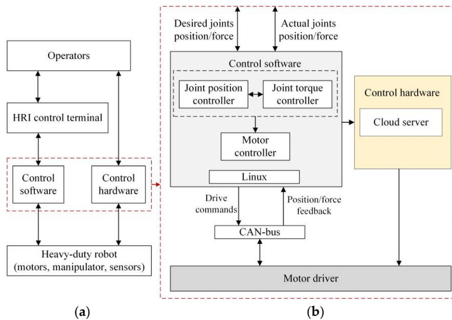
**Figure 1.** (a) The heavy-duty robot system component; (b) Control system.
