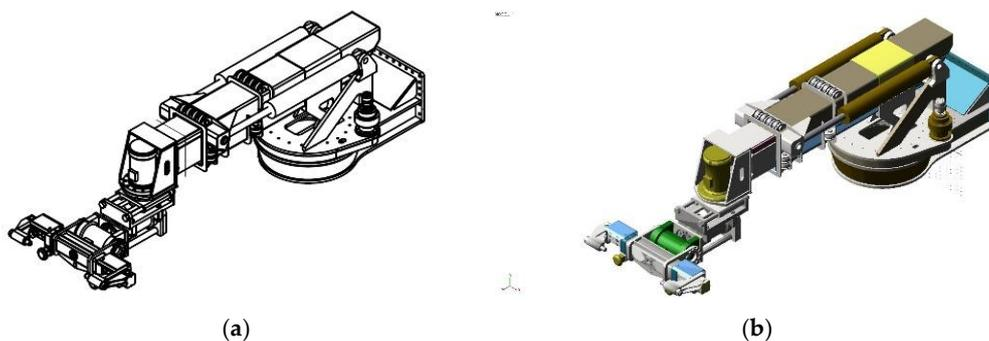
Figure 5. (a) Heavy-duty manipulator; (b) Adams dynamic model.
