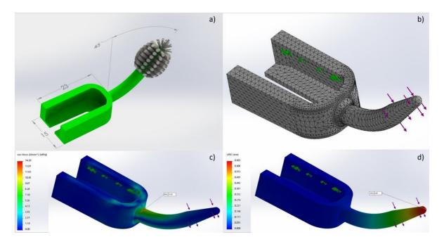
**Figure 2.** (a) Cleft Toothbrush—3D model; (b) finite elements solid mesh; (c) results of the stress in the Cleft Toothbrush due to the applied load (maximum of 14.20 MPa at the connection between the horn and the body); and (d) the maximum displacement of the adapter due to the applied load—0.663 mm reached in the tip (red area).
