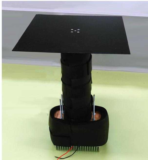
**Figure 6.** Prototype of the TEG solar flat panel with buried heat sink.
