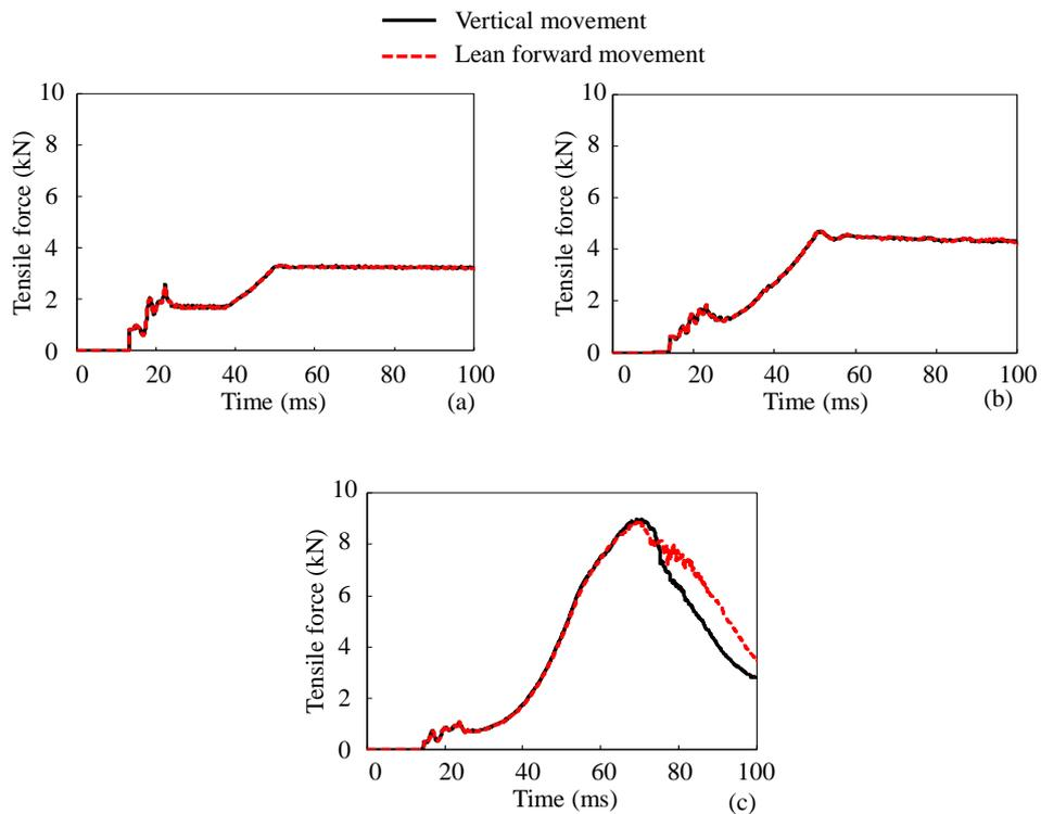
**Figure 14.** Time histories of the tensile forces on the (a) retractor belt, (b) shoulder belt, and (c) lap belt.
