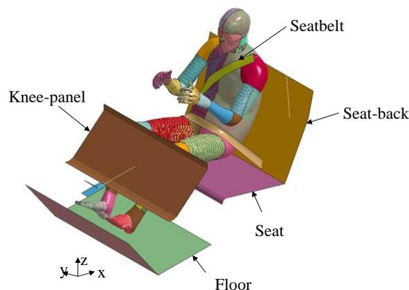
**Figure 3.** Anthropomorphic 50th percentile male total human model for safety ver.4 (AM50 human model) [10] seated in the vehicle cabin model [12].
