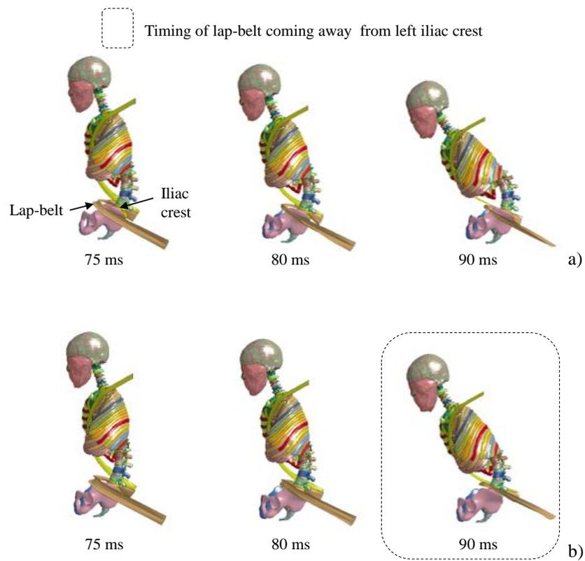
**Figure 11.** Dynamic behavior of the lap belt under two seat conditions (view from left): (a) vertical seat movement and (b) lean forward seat movement.
