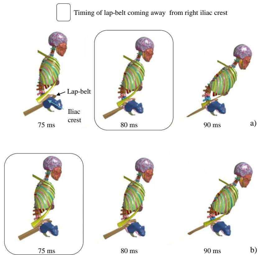
**Figure 12.** Dynamic behavior of the lap belt under two seat conditions (view from right): (a) vertical seat movement and (b) lean forward seat movement.
