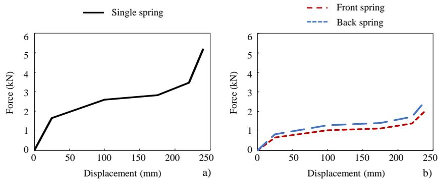
**Figure 5.** Force-displacement characteristics used in the spring models of the seats: (a) vertical seat movement and (b) lean forward seat movement.
