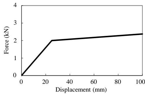
**Figure 6.** Force-displacement characteristics used in the spring models in the knee panels.
