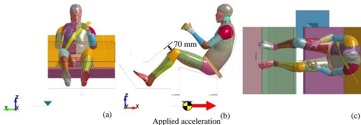
**Figure 8.** Vehicle cabin and AM50 human models from (a) front, (b) side, and (c) top views.
