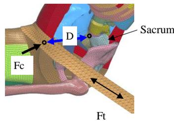
**Figure 16.** Illustration of the resultant contact force (Fc) between lap belt and abdomen, deformation of the abdomen (D), and tensile force of the lap belt (Ft).
