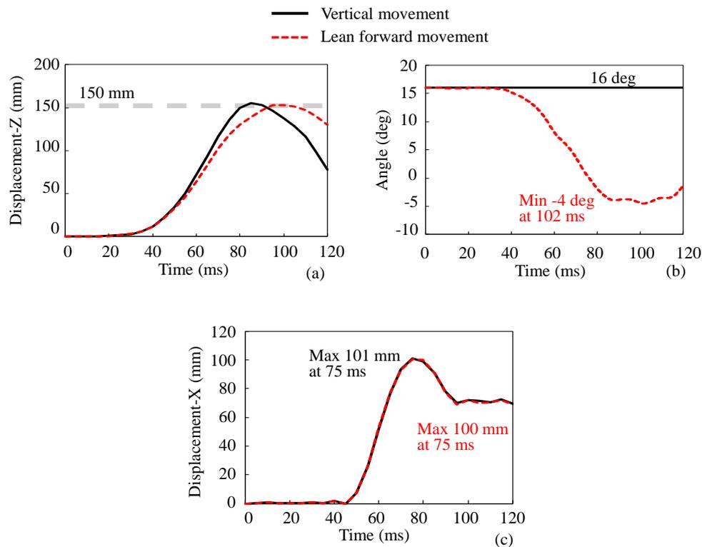
**Figure 13.** Time histories of (a) seat height, (b) seat angle, and (c) knee-panel displacement under two seat conditions.
