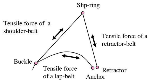
Figure 9. Tensile force activated on various restraining belts.
