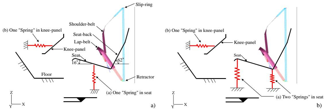
**Figure 4.** Vehicle cabin model and modified spring model used in this study: (a) vertical seat movement and (b) lean forward seat movement.
