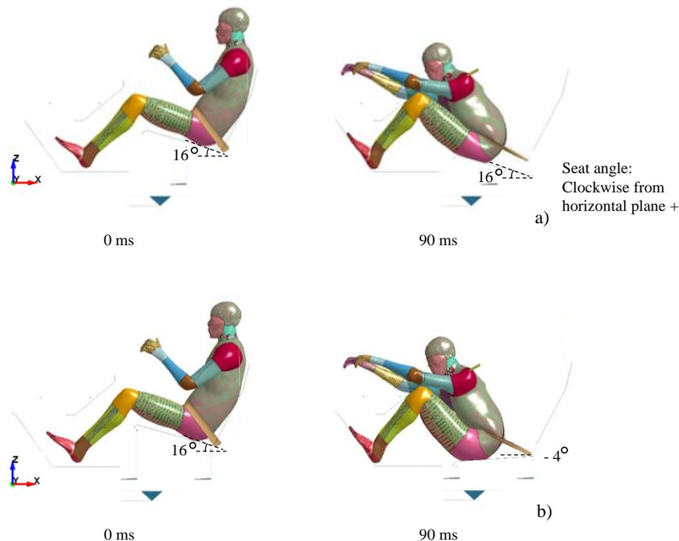
Figure 10. Dynamic behaviors of AM50 dummies under two seat conditions: (a) vertical seat movement and (b) lean forward seat movement.
