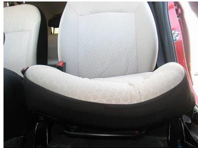
**Figure 2.** Photograph of residual deformation of the front passenger seat in a car after a Japan new car assessment program (JNCAP) full frontal rigid barrier impact test.
