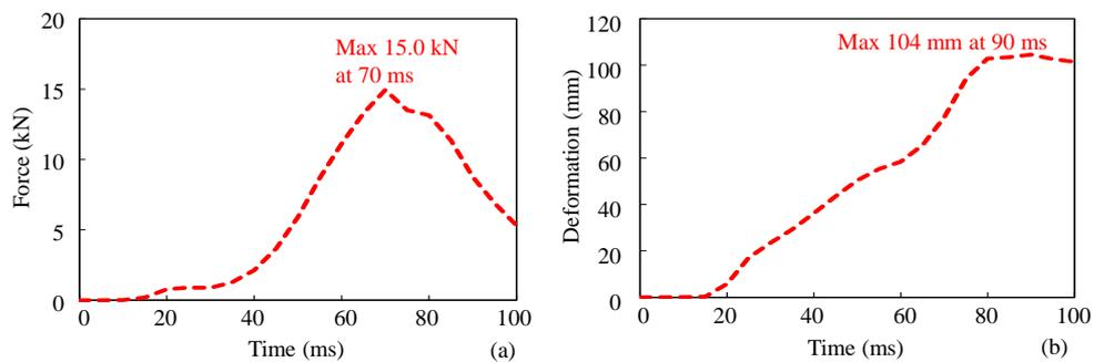
**Figure 17.** Time history of (a) resultant contact force (Fc) and (b) deformation of the abdomen (D) under lean forward movement conditions.
