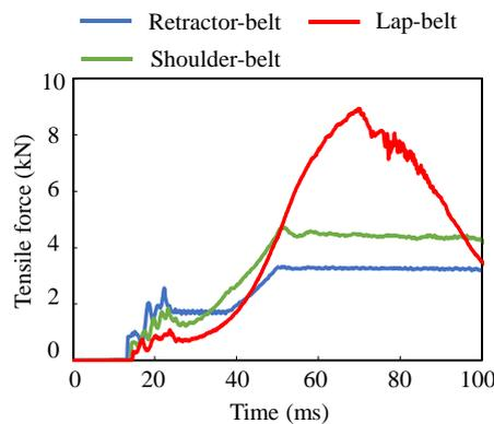
**Figure 15.** Time history of tensile forces of the seatbelt under the lean forward movement seat condition.
