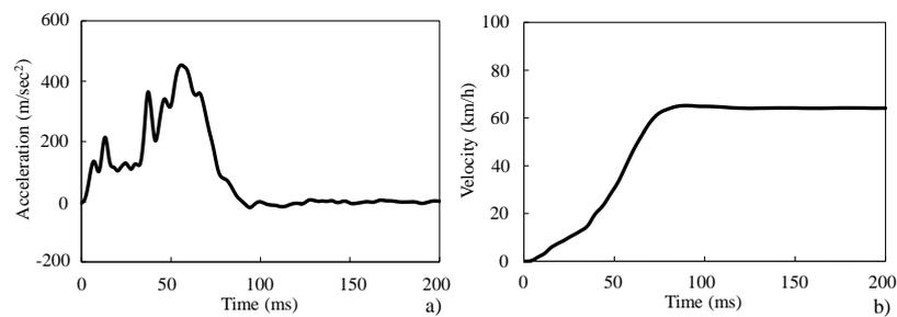
**Figure 7.** Time-series of (a) acceleration and (b) velocity applied to the vehicle cabin model.
