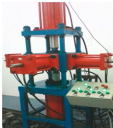
**Figure 1.** Self-developed true triaxial test machine.
