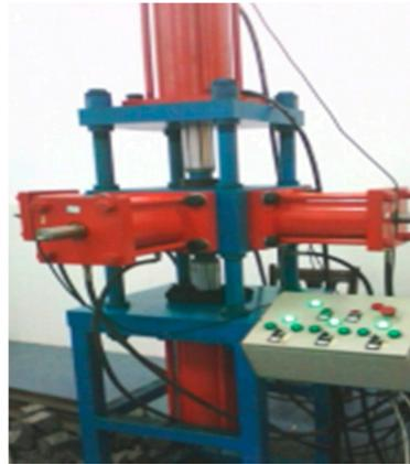
**Figure 1.** Self-developed true triaxial test machine.
