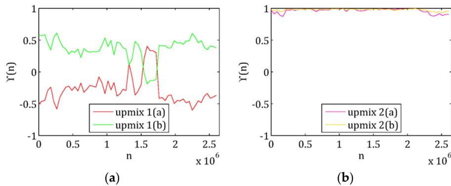
**Figure 11.** Correlation degree of surround channels: (a) Upmix 1(a) and 1(b); (b) upmix 2(a) and 2(b).
