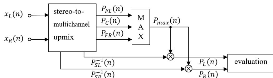
**Figure 6.** Block diagram: Power test.
