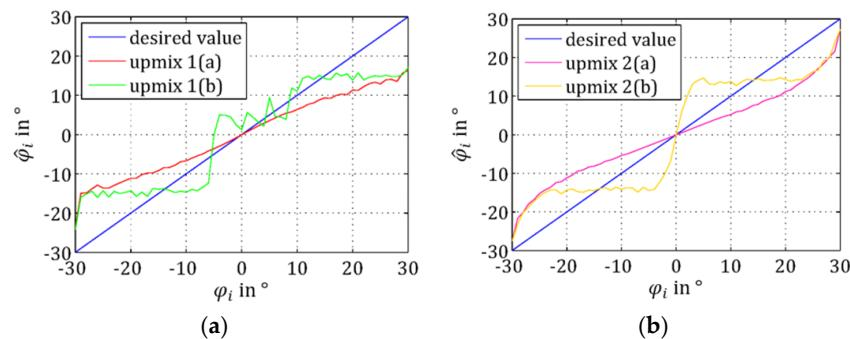
**Figure 3.** Panning test—angle of the virtual test sound sources compared with the determined virtual sound sources of the upmix algorithms: (a) algorithms upmix 1(a) and 1(b); (b) algorithms upmix 2(a) and 2(b).
