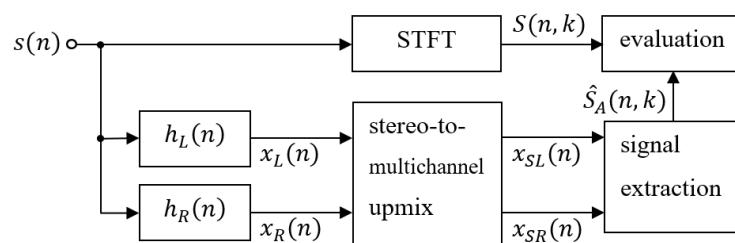
**Figure 4.** Block diagram: Direct signal test. Note that this is a simplified illustration of room impulse responses as a summary. See Appendix A for details of used room impulse responses and the calculation of  $x_L$  and  $x_R$ . STFT: short-time Fourier transform.
