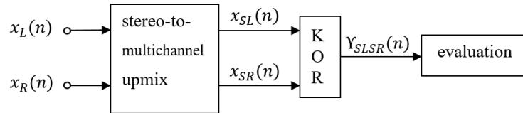
**Figure 10.** Block diagram: Phase test. Correlation degree is calculated in the block “KOR”.
