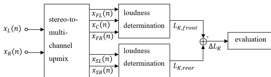
**Figure 8.** Block diagram: Loudness test.
