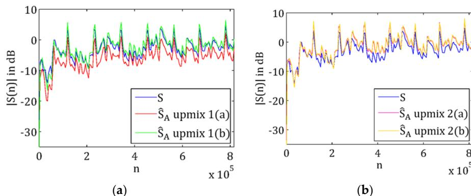
**Figure 5.** Direct signal test—remaining surround channel direct signal: (a) Algorithms upmix 1(a) and 1(b); (b) algorithms upmix 2(a) and 2(b). Note that the index  $n$  in the plots represents discrete values of time.  $|S(n)|$  represents the magnitude of the respective complex direct signal averaged over all frequencies.
