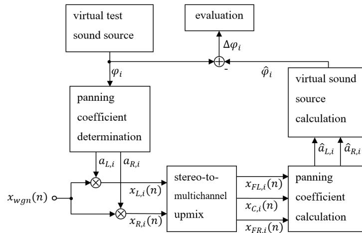
**Figure 2.** Block diagram: Time- and frequency-independent panning test.
