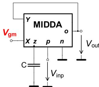
**Figure 8.** Simple application of a proposed MIDDDA in a first-order high-pass filter with adjustable pole frequency.
