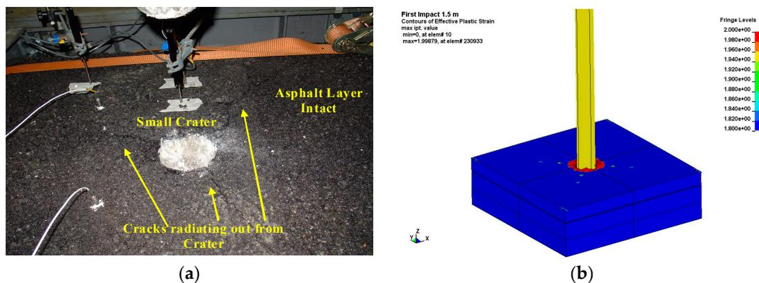
**Figure 17.** Damage of the multi-layer slab after the first impact: (a) damage pattern of slab in the laboratory test; (b) damage pattern of slab in the numerical simulation.
