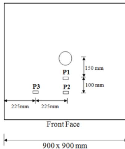
**Figure 14.** Positioning of the potentiometers.
