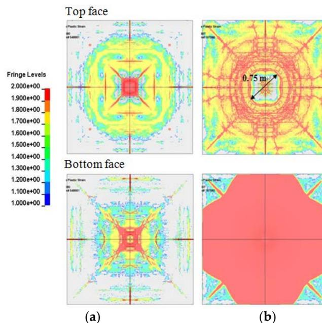
**Figure 12.** Damage contour for the AC and HSC layer in the multi-layers pavement: (a) damage contour of the AC layer in the numerical simulation; (b) damage contour of the HSC layer in the numerical simulation.
