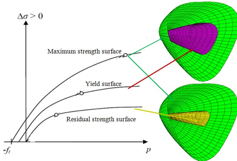
**Figure 1.** Strength surfaces for the Karagozian and Case concrete model (KCC) material model [14].
