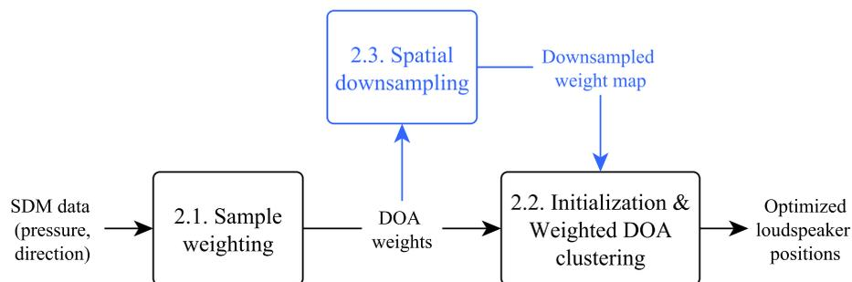
**Figure 1.** Position optimization system outline. Spatial Decomposition Method (SDM) generated data containing directions of arrival (DOA) the omnidirectional pressure values for each sample are provided to the algorithm, from which the optimized loudspeaker positions are approximated. The numbers inside the boxes refer to the corresponding sections in this paper, spatial downsampling part (in blue) working as an extra acceleration component for the main algorithm (in black).
