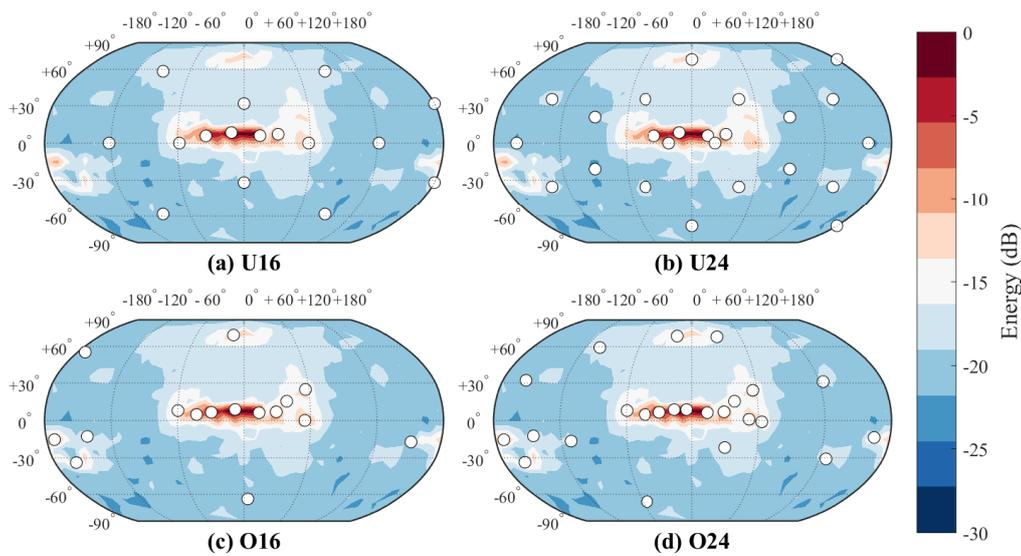
**Figure 4.** Loudspeaker setups used in the concert hall samples: (a) uniform setup with 16 loudspeakers; (b) uniform setup with 24 loudspeakers; (c) optimized setup with 16 loudspeakers; and (d) optimized setup with 24 loudspeakers.
