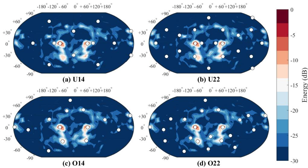
**Figure 3.** Loudspeaker setups (white circles) overlaid with the spatial map of overall sound energy in the small room case: (a) uniform setup with 14 loudspeakers; (b) uniform setup with 22 loudspeakers; (c) optimized setup with 14 loudspeakers; and (d) optimized setup with 22 loudspeakers.
