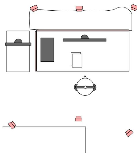
**Figure 2.** A sketch of the listening test setup. The listener (in the middle) is surrounded by six infrared cameras (red) that track the movements of the noise-canceling headphones. The field of view has been obscured with a curtain.
