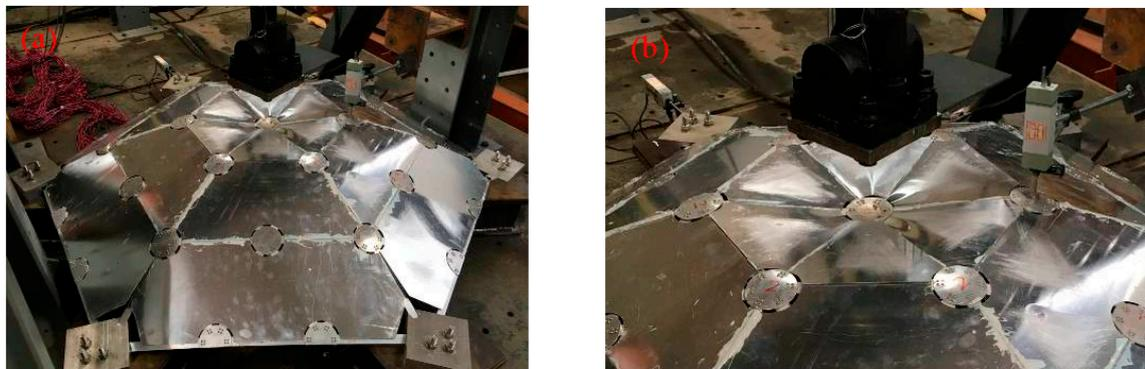
**Figure 5.** Failure modes of the combined lattice shell model: (a) The overall failure profile; (b) The amplified profile of a local destabilization area.
