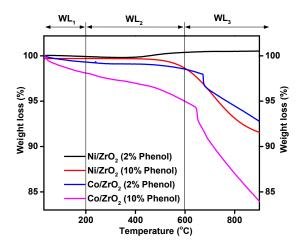
**Figure 16.** TGA profile of used Ni/ZrO<sub>2</sub> and Co/ZrO<sub>2</sub> catalysts.
