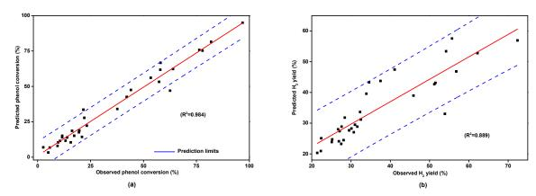
**Figure 8.** Parity charts of predicted versus observed responses for the reduced models of phenol conversion  $(Y_1)$  (**a**) and hydrogen yield  $(Y_2)$  (**b**) with a 95% prediction band.
