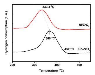
**Figure 3.** TPR-H<sub>2</sub> profiles for the Ni/ZrO<sub>2</sub> and Co/ZrO<sub>2</sub> catalysts.
