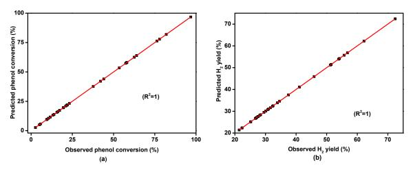
**Figure 6.** Parity charts of predicted versus observed responses for the initial models of (**a**) phenol conversion  $(Y_1)$  and (**b**) hydrogen yield  $(Y_2)$ , including all main and interaction independent variables.
