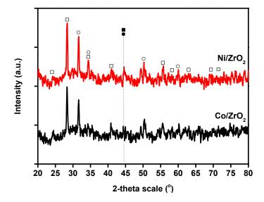
**Figure 2.** XRD pattern for Ni/ZrO<sub>2</sub> and Co/ZrO<sub>2</sub> catalysts after reduction at 600  $^{\circ}$ C; (●) peaks correspond to metallic Ni, (■) peaks correspond to metallic Co, (□) peaks correspond to monoclinic phase of ZrO<sub>2</sub> (m-ZrO<sub>2</sub>) and (○) peaks correspond to tetragonal phase of ZrO<sub>2</sub> (t-ZrO<sub>2</sub>).
