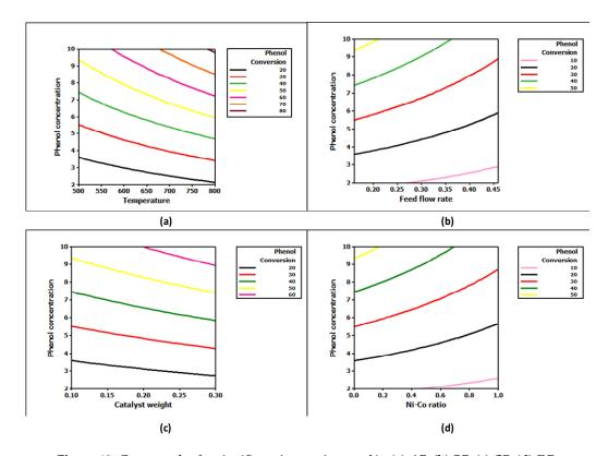
**Figure 12.** Contour plot for significant interactions on  $Y_1$ : (a) AE; (b) BE; (c) CE; (d) DE.
