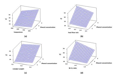
**Figure 13.** Surface plot for significant interactions on  $Y_2$ : (a) AE; (b) BE; (c) CE; (d) DE.
