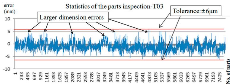
Figure 22. Statistics of parts inspection for T03.
