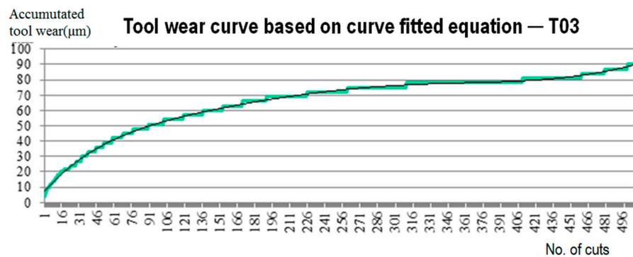
Figure 14. Tool wear curve for T03.
