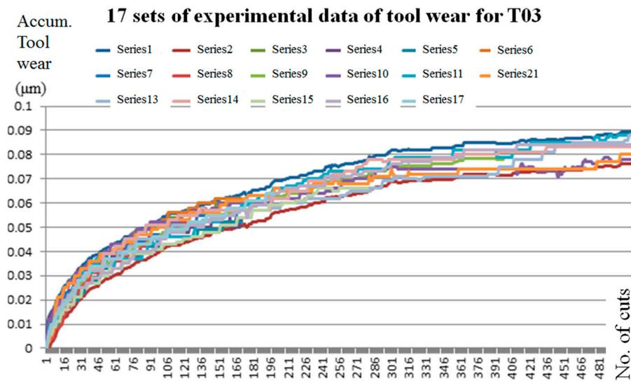
Figure 12. Statistics of tool wear for T03.
