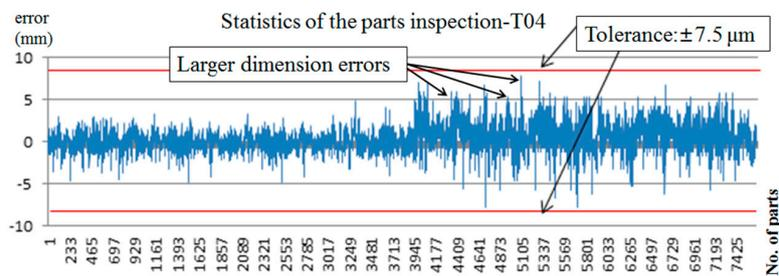
Figure 23. Statistics of parts inspection for T04.
