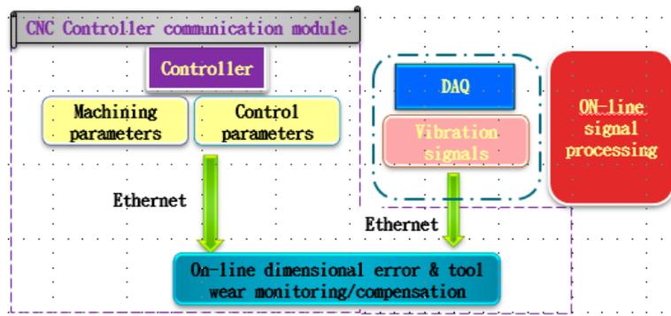
Figure 16. The communication module extracts information for monitoring/compensation.
