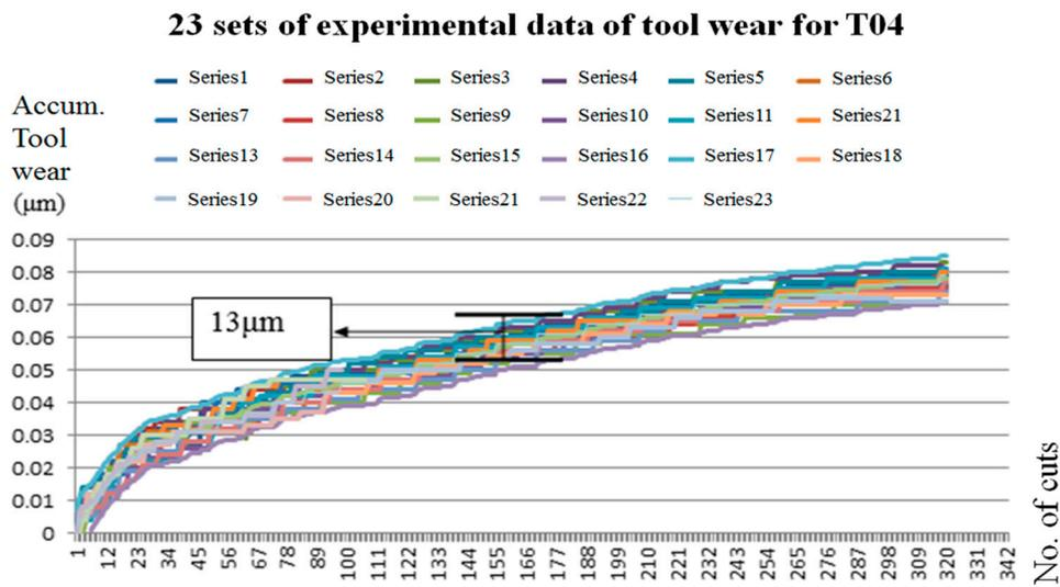
Figure 13. Statistics of tool wear for T04.
