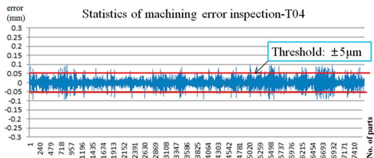
**Figure 21.** On-machine machining inspection result for T04.
