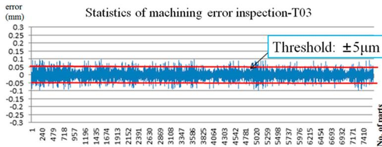
**Figure 20.** On-machine machining inspection result for T03.
