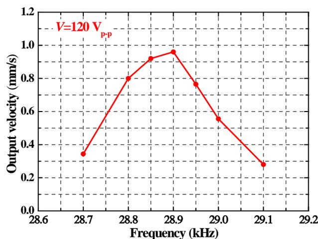
Figure 9. Frequency characteristics of the screw-type piezoelectric ultrasonic motor.
