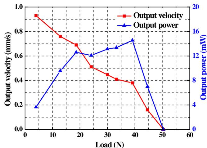
**Figure 11.** Load characteristics of the screw-type piezoelectric ultrasonic motor.
