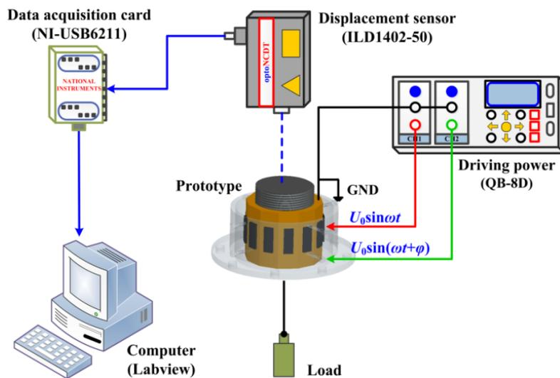
Figure 8. Schematic drawing of the experiment system.
