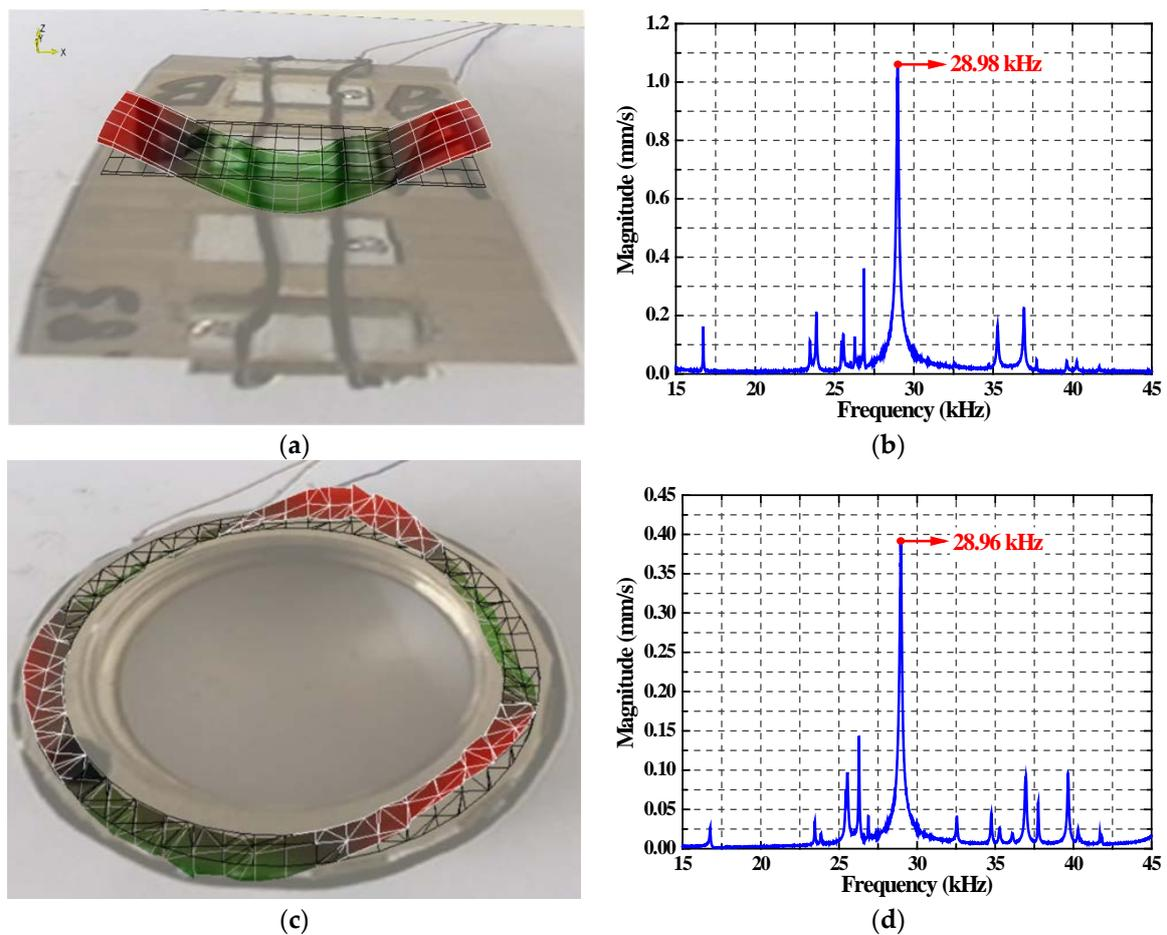
**Figure 7.** Vibration testing result of the motor under the exciting group B: (a) axial vibration mode shape; (b) axial vibration velocity response spectrum; (c) circumferential vibration mode shape; (d) circumferential vibration velocity response spectrum.
