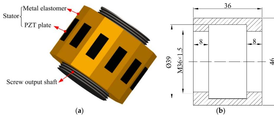
**Figure 1.** Structure of the proposed piezoelectric ultrasonic motor: (a) the three-dimensional model of the motor; (b) the main structure parameters of the stator (unit: mm).
