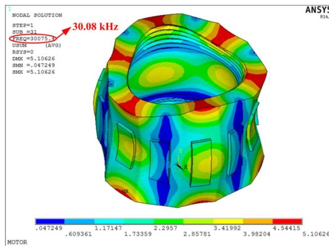
**Figure 3.** Working modal shape of the stator by Finite Element Method (FEM).
