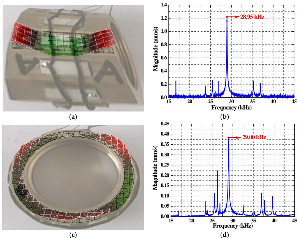
**Figure 6.** Vibration testing result of the motor under the exciting group A: (a) axial vibration mode shape; (b) axial vibration velocity average response spectrum; (c) circumferential vibration mode shape; (d) circumferential vibration velocity average response spectrum.
