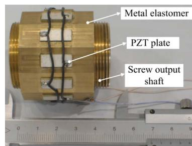
Figure 5. Prototype of the proposed piezoelectric ultrasonic motor.
