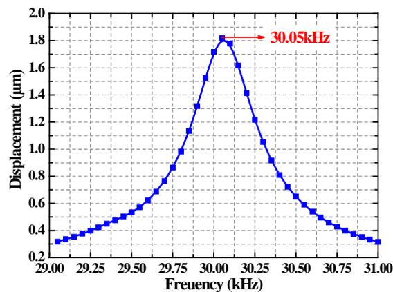
Figure 4. Simulation result: The relationship between frequency and displacement of a particle.
