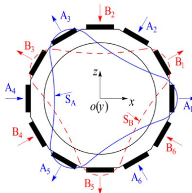
**Figure 2.** The three-wavelength exciting mode of the proposed piezoelectric ultrasonic motor.
