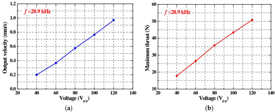
**Figure 10.** Voltage characteristics of the screw-type piezoelectric ultrasonic motor: (a) the relationship between the driving voltages and the output velocities; (b) the relationship between the driving voltages and the maximum thrust.
