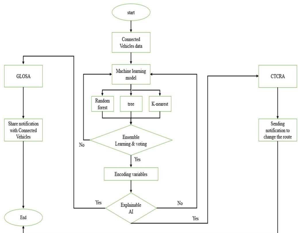
Figure 12. Algorithm improving driving style in connected vehicles (IDSCV).
