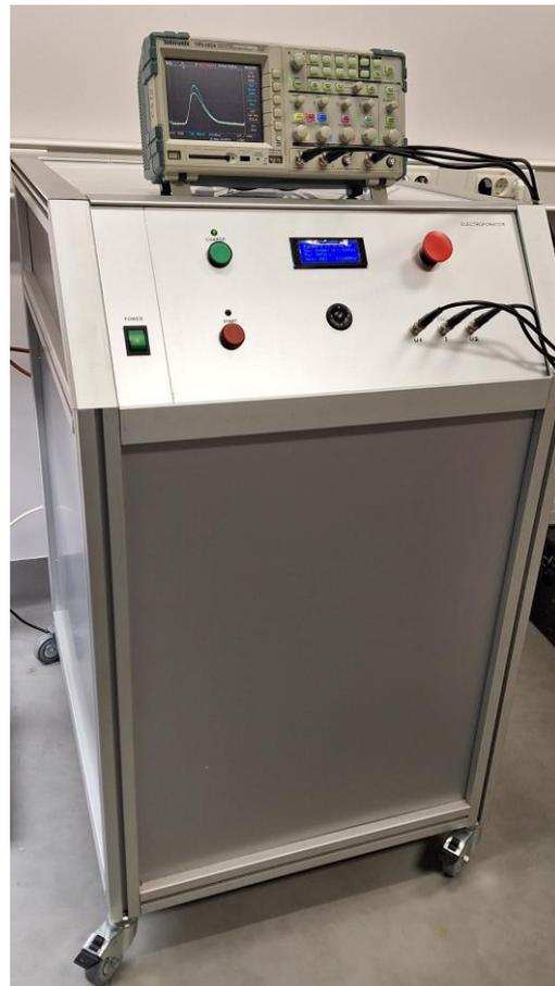
**Figure 3.** A photo of the developed two-range, 12-stage Marx generator. The oscilloscope is used to measure voltage and current pulses.
