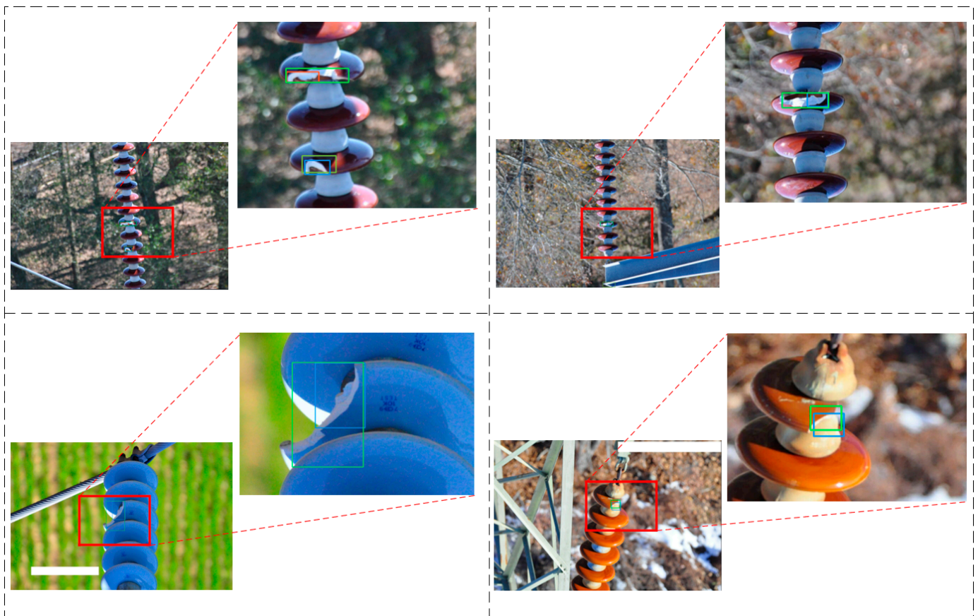
Figure 5. Redundant prediction boxes in insulator defect instance segmentation.
