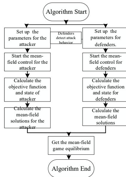
Figure 2. The procedure of the mean-field game algorithm.
