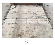
**Figure 8.** Expansion process of concrete cracks at the old and new interfaces of wet joints. (a) Initial cracking of concrete at the old/new interface of wet joints. (b) Expansion of concrete cracks at the old and new interfaces of wet joints. (c) Cracking of concrete slabs.
