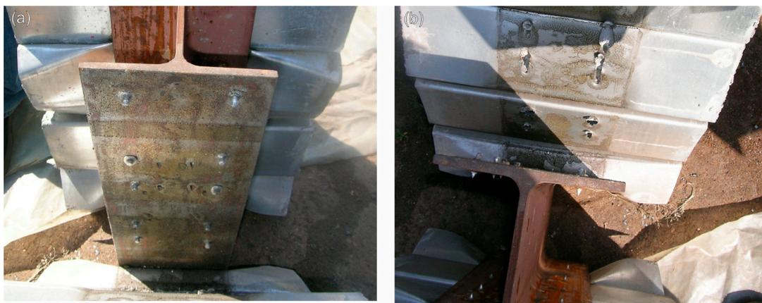
**Figure 10.** Failure of specimen from model no. 2 (consisted of 1.00 mm thick metal sheet and 4 shot nails) after separating concrete slab from steel beam: (a) steel beam view; and (b) corrugated sheet view.
