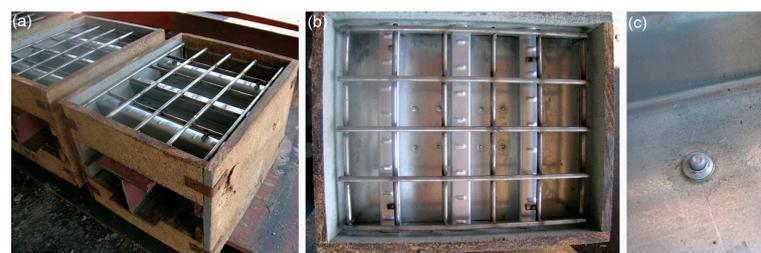
Figure 5. Samples prepared for concreting slabs in a horizontal position: (a) view; (b) view of the corrugation sheet and reinforcement; and (c) view of nail driven into the sheet.
