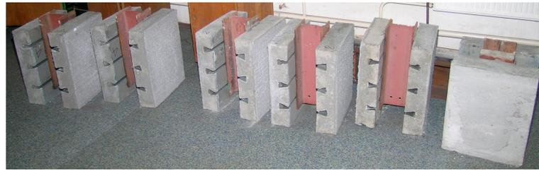
**Figure 6.** Samples for push-out tests.
