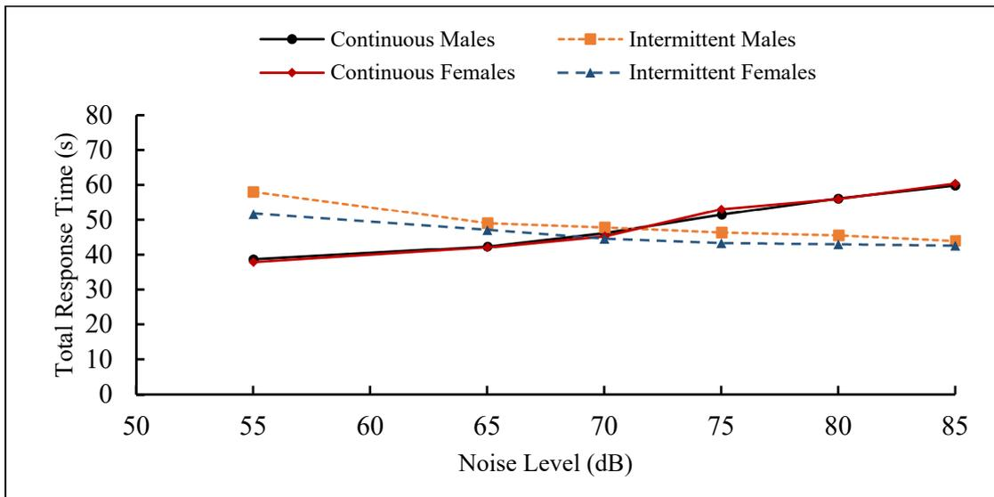
Figure 4. Relationship between total response time on continuous and intermittent noise levels.
