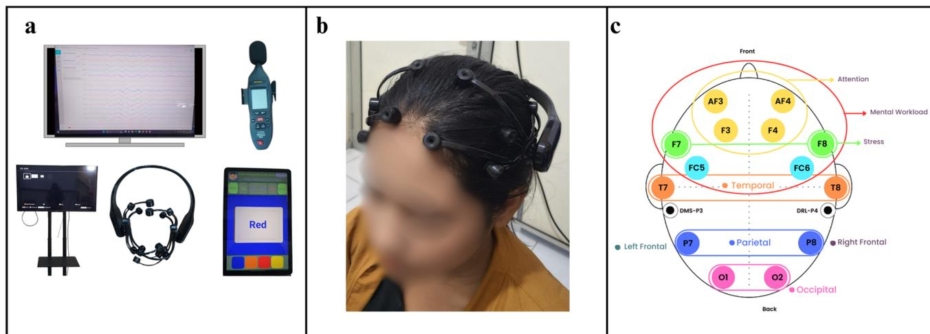
**Figure 2.** (a) Equipment of the EEG Experiment; (b) An actual photograph showing the experimental setup in the laboratory; (c) Electrode placement on the Emotiv Epoch.
