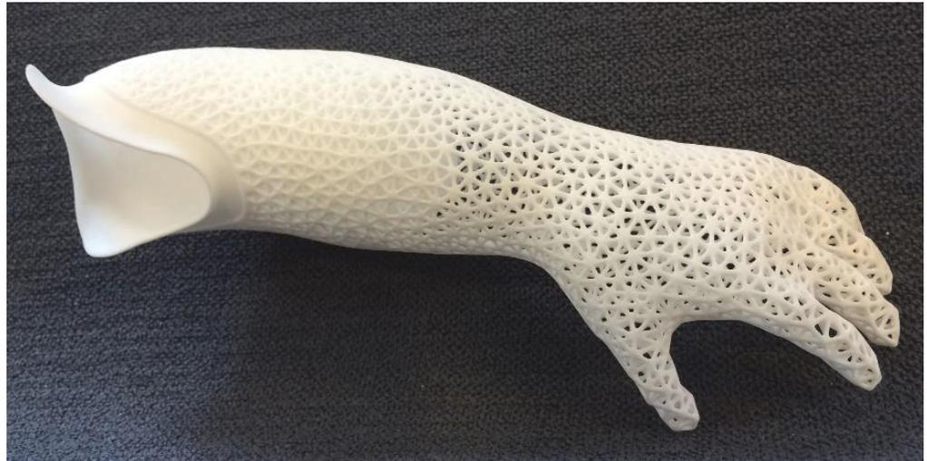
**Figure 5.** 3D printed prosthetic socket and arm produced using PBF.
