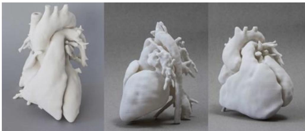
**Figure 4.** Heart models manufactured via 3D-printing SLA method [13].
