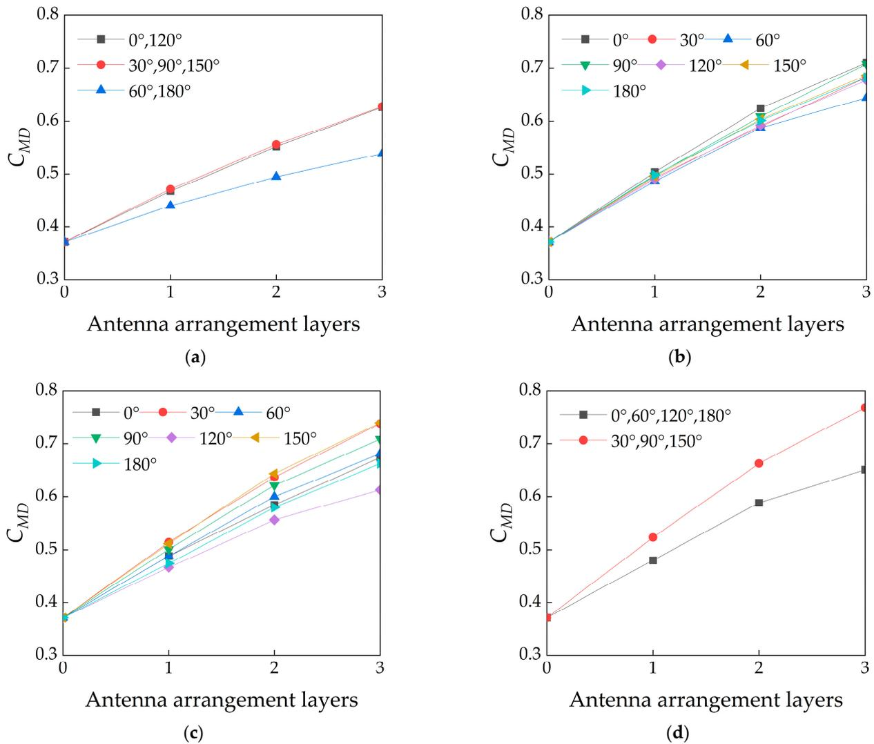
**Figure 21.** Variation curve of windward base overturning moment coefficient of telecommunication tower with antenna arrangement layers. (a) Three antennas per layer. (b) Four antennas per layer. (c) Five antennas per layer. (d) Six antennas per layer.
