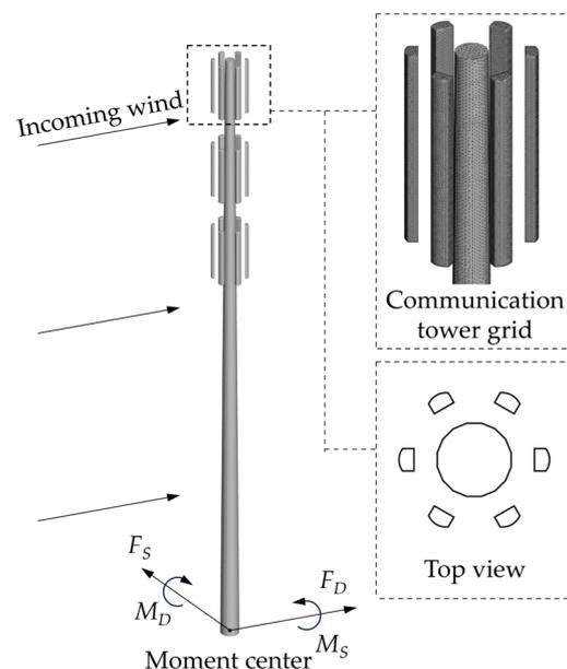
**Figure 1.** Schematic of the telecommunication tower mesh and wind loads [31].
