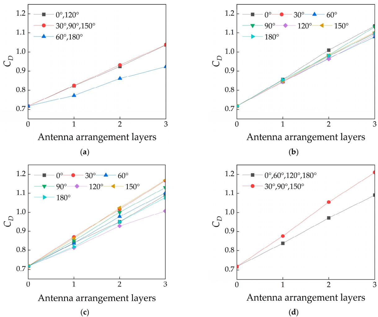
**Figure 20.** Variation curve of drag coefficient of telecommunication tower with antenna arrangement layers. (a) Three antennas per layer. (b) Four antennas per layer. (c) Five antennas per layer. (d) Six antennas per layer.
