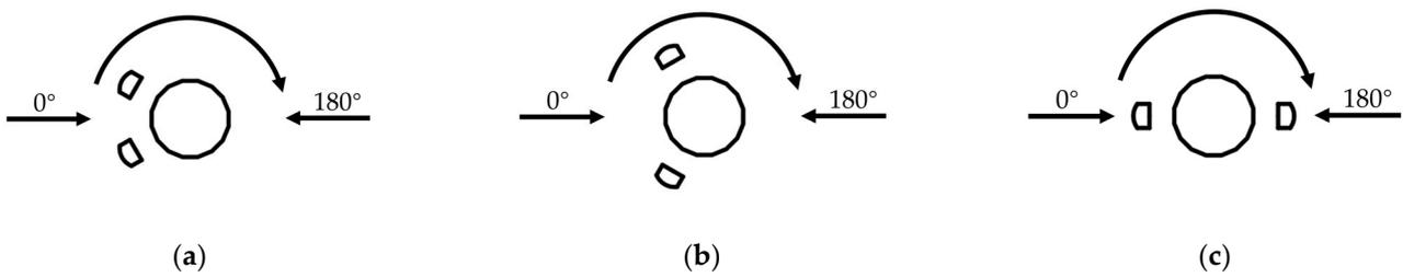
Figure 8. Arrangement form when 2 antennas are deployed. (a) Form 1. (b) Form 2. (c) Form 3.
