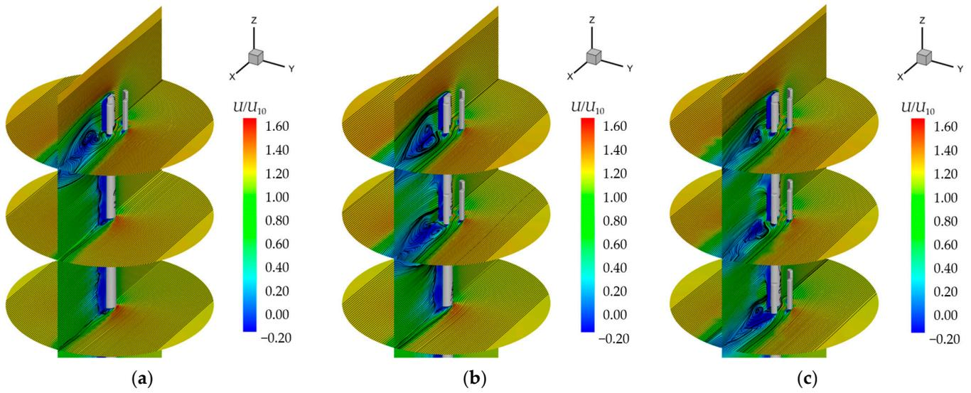
**Figure 27.** The flow field around the telecommunication tower with 6 antennas per layer, at a wind direction of 30°. (a) One layer of antennas. (b) Two layers of antennas. (c) Three layers of antennas.
