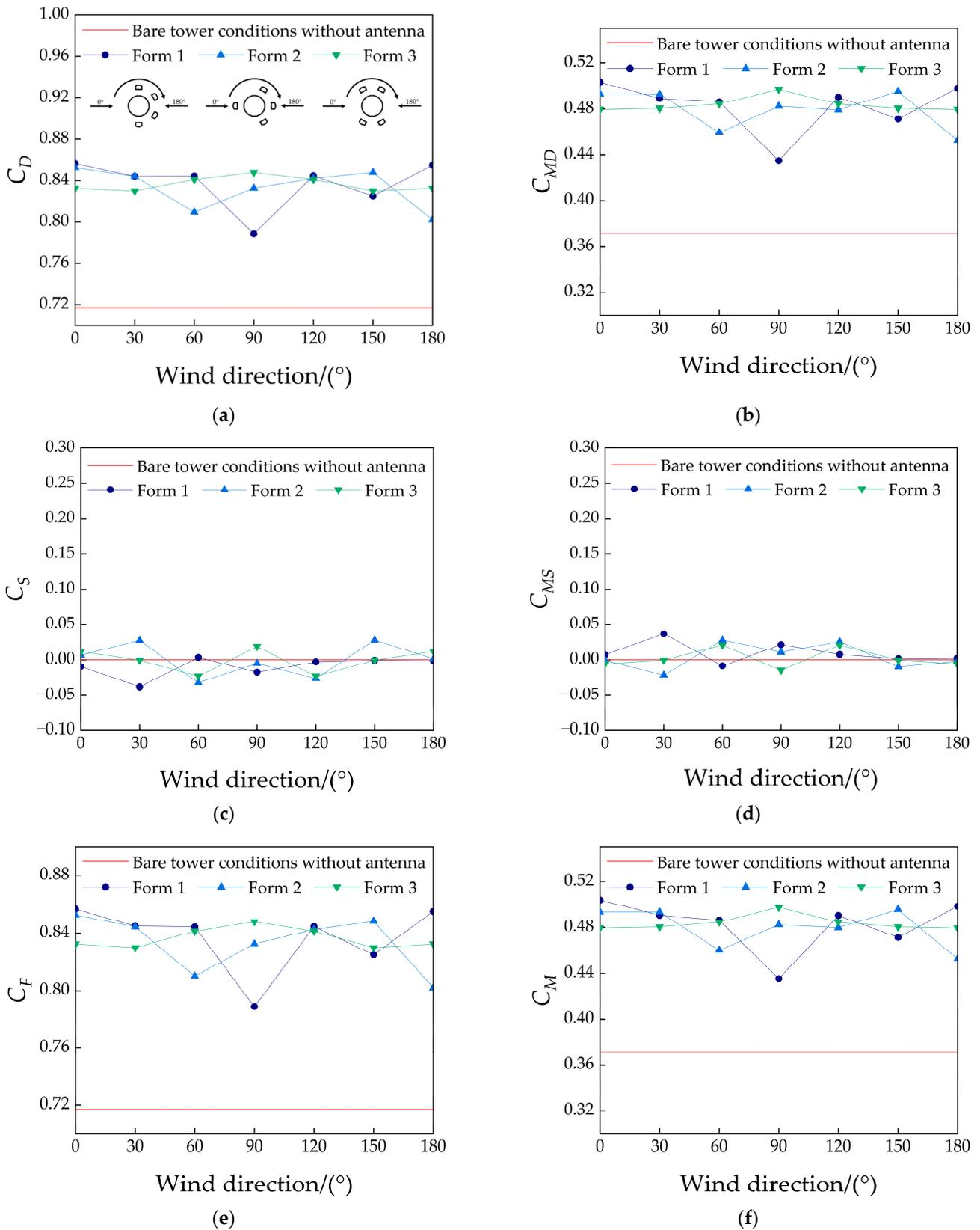
**Figure 13.** Variation curve of wind load on the telecommunication tower with wind direction when 4 antennas are arranged. (a) Drag coefficient. (b) Windward base overturning moment coefficient. (c) Lateral force coefficient. (d) Crosswind base overturning moment coefficient. (e) Overturning force coefficient. (f) Overturning moment coefficient.
