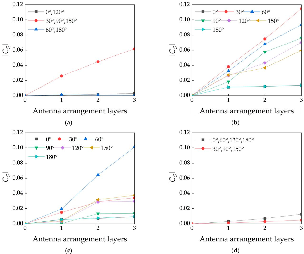
**Figure 22.** Variation curve of lateral force coefficient of telecommunication tower with antenna arrangement layers. (a) Three antennas per layer. (b) Four antennas per layer. (c) Five antennas per layer. (d) Six antennas per layer.
