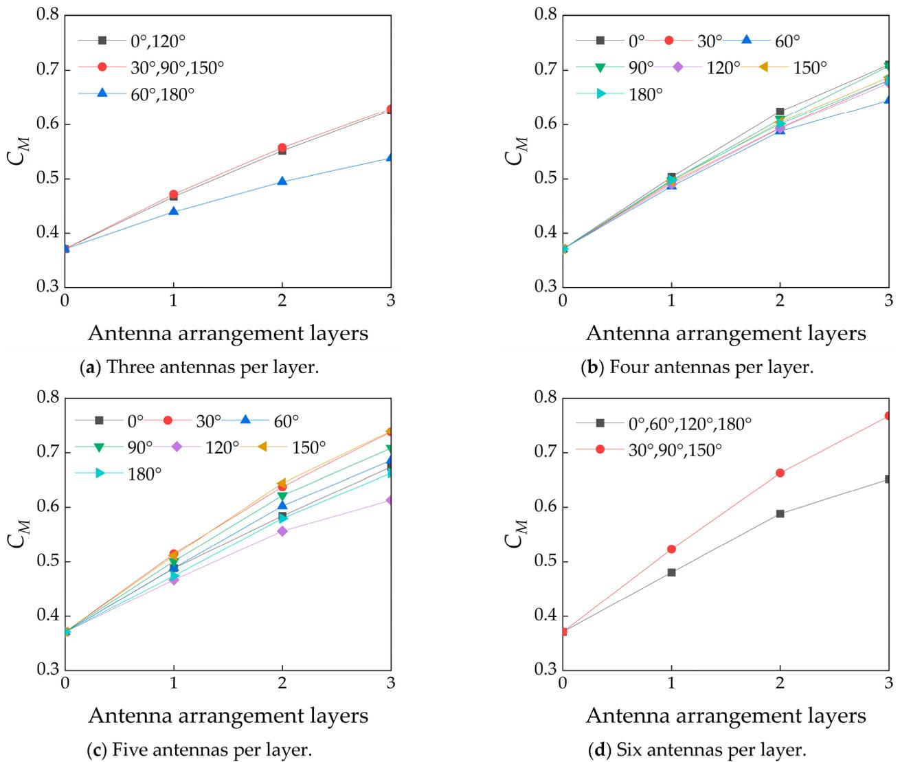
**Figure 25.** Variation curve of overturning moment coefficient of telecommunication tower with antenna arrangement layers. (a) Three antennas per layer. (b) Four antennas per layer. (c) Five antennas per layer. (d) Six antennas per layer.
