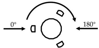
Figure 6. Arrangement form when 3 antennas are deployed.
