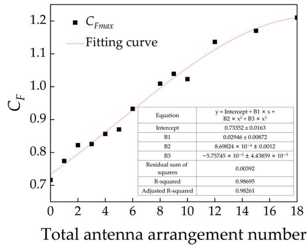
Figure 28. Curve of the maximum overturning force coefficient variation with the total antenna arrangement number.
