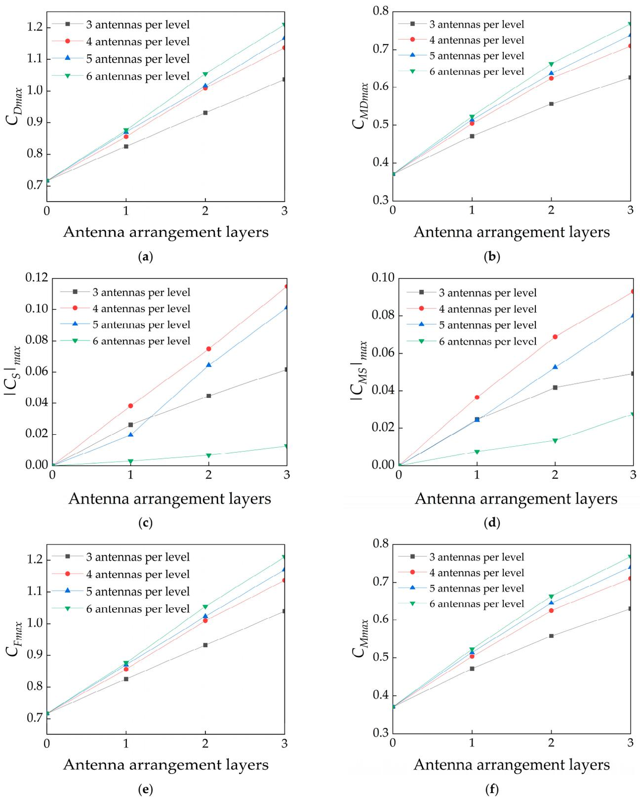
**Figure 26.** Influence of the antenna arrangement layers on the wind load of the telecommunication tower. (a) Drag coefficient. (b) Windward base overturning moment coefficient. (c) Lateral force coefficient. (d) Crosswind base overturning moment coefficient. (e) Overturning force coefficient. (f) Overturning moment coefficient.
