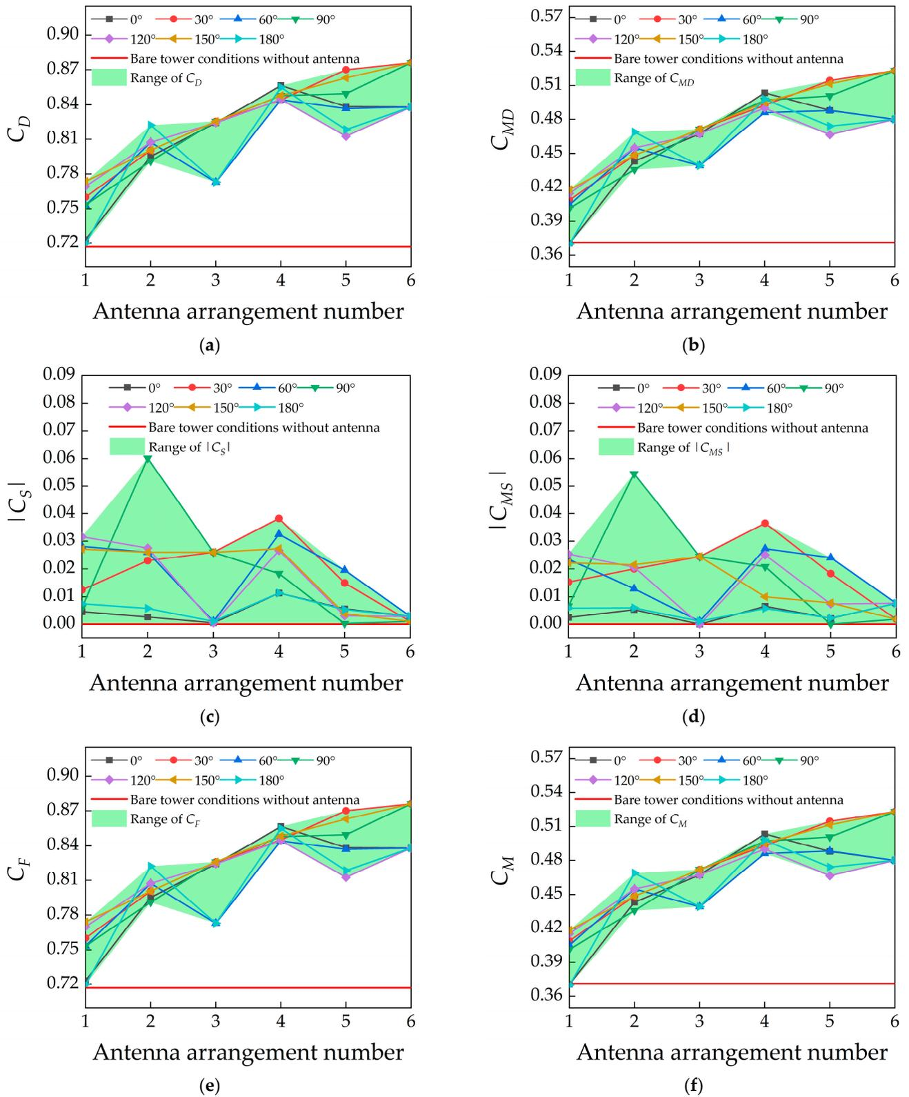
**Figure 15.** Impact of single-layer antenna arrangement on the wind load of telecommunication towers. (a) Drag coefficient. (b) Windward base overturning moment coefficient. (c) Lateral force coefficient. (d) Crosswind base overturning moment coefficient. (e) Overturning force coefficient. (f) Overturning moment coefficient.
