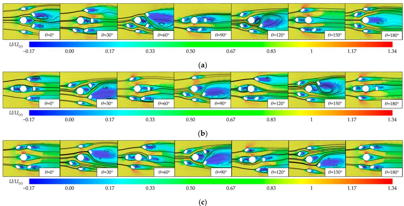
**Figure 14.** Velocity contour and streamline diagram at the mid-height cross-section of the antennas when 4 antennas are arranged. (a) Form 1. (b) Form 2. (c) Form 3.
