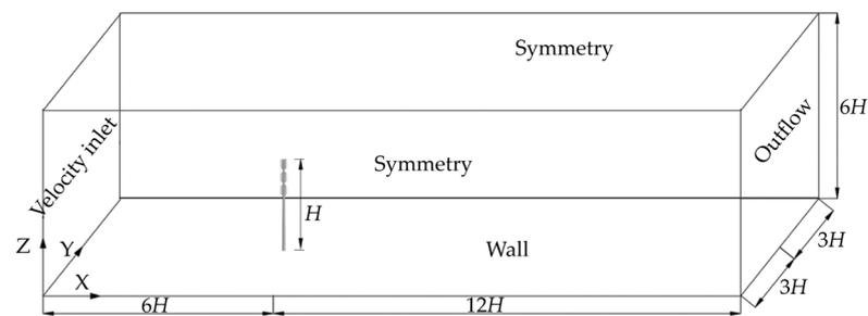
**Figure 2.** Diagram of the computational domain dimensions.
