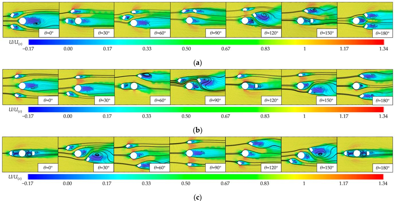
**Figure 12.** Velocity contour and streamline diagram at the mid-height cross-section of the antennas when 2 antennas are arranged. (a) Form 1. (b) Form 2. (c) Form 3.
