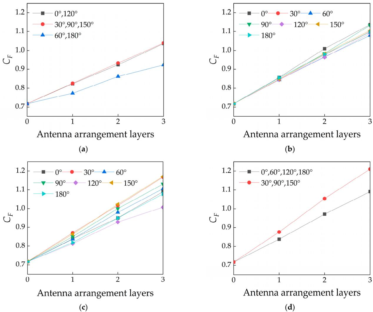
**Figure 24.** Variation curve of overturning force coefficient of telecommunication tower with antenna arrangement layers. (a) Three antennas per layer. (b) Four antennas per layer. (c) Five antennas per layer. (d) Six antennas per layer.
