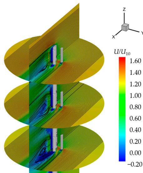
**Figure 19.** Flow field around the telecommunication tower with 3 layers of antennas, 4 antennas per layer arranged in form 1, at a wind direction of  $0^\circ$ .
