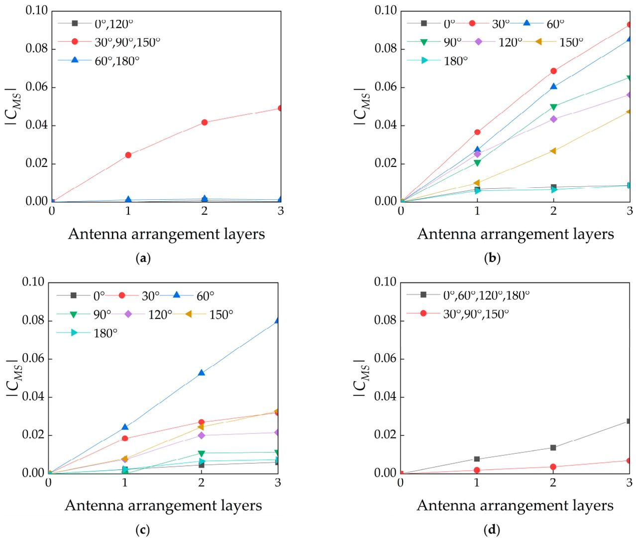
**Figure 23.** Variation curve of crosswind base overturning moment coefficient of telecommunication tower with antenna arrangement layers. (a) Three antennas per layer. (b) Four antennas per layer. (c) Five antennas per layer. (d) Six antennas per layer.
