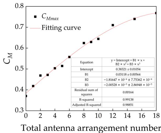
Figure 29. Curve of the maximum overturning moment coefficient variation with the total antenna arrangement number.
