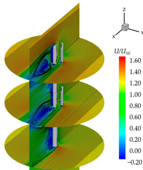
**Figure 18.** Flow field around the telecommunication tower with 2 layers of antennas, 6 antennas per layer, at a wind direction of  $30^\circ$ .
