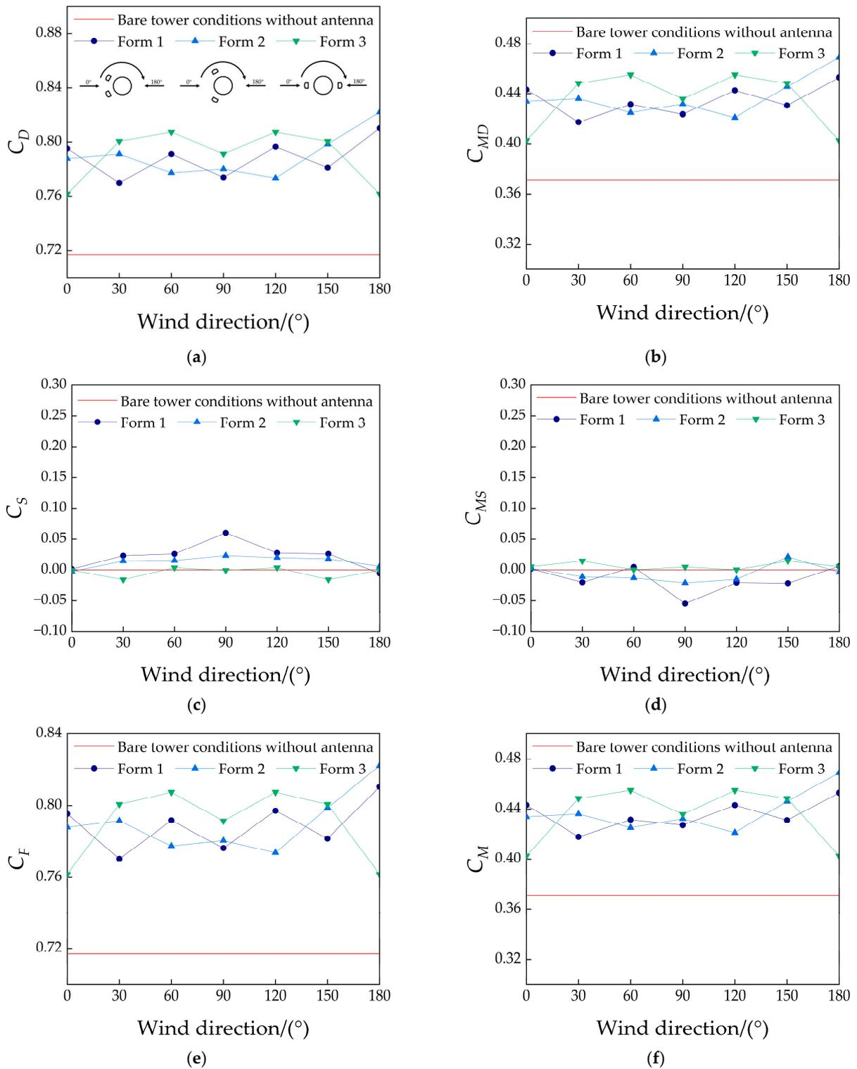
**Figure 11.** Variation curve of wind load on the telecommunication tower with wind direction when 2 antennas are arranged. (a) Drag coefficient. (b) Windward base overturning moment coefficient. (c) Lateral force coefficient. (d) Crosswind base overturning moment coefficient. (e) Overturning force coefficient. (f) Overturning moment coefficient.
