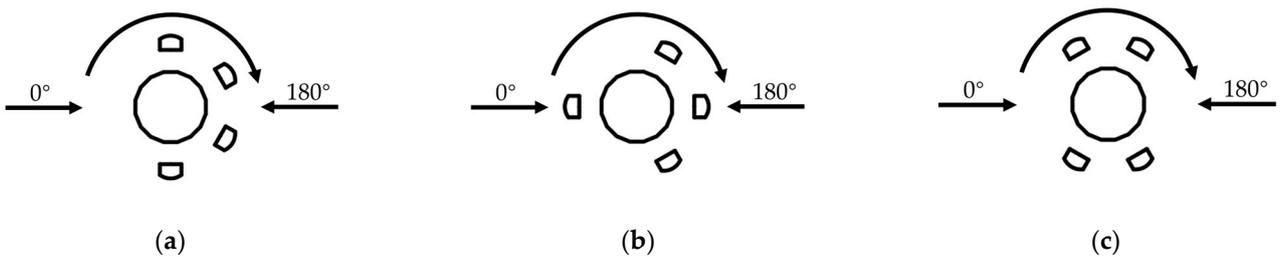
Figure 9. Arrangement form when 4 antennas are deployed. (a) Form 1. (b) Form 2. (c) Form 3.
