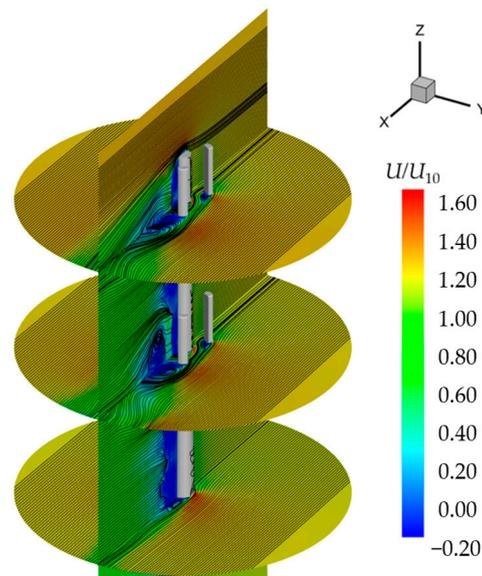
**Figure 17.** Flow field around the telecommunication tower with 2 layers of antennas, 3 antennas per layer, at a wind direction of  $30^\circ$ .
