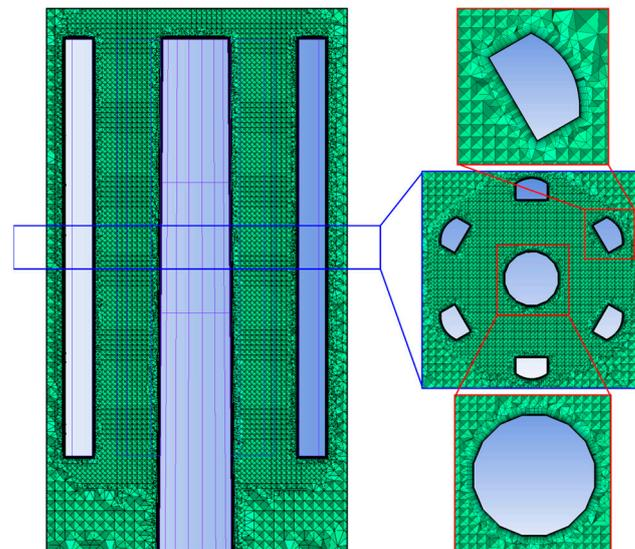
**Figure 4.** Mesh around the tower cylinder and antennas.
