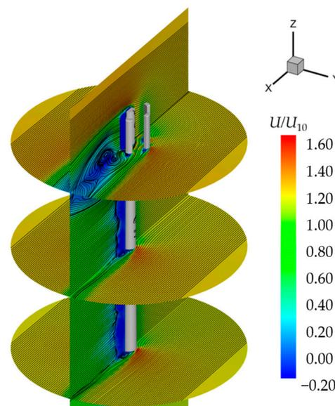
**Figure 16.** Flow field around the telecommunication tower with 1 layer of antennas, 6 antennas per layer, at a wind direction of  $30^\circ$ .
