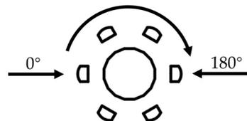
Figure 7. Arrangement form when 6 antennas are deployed.
