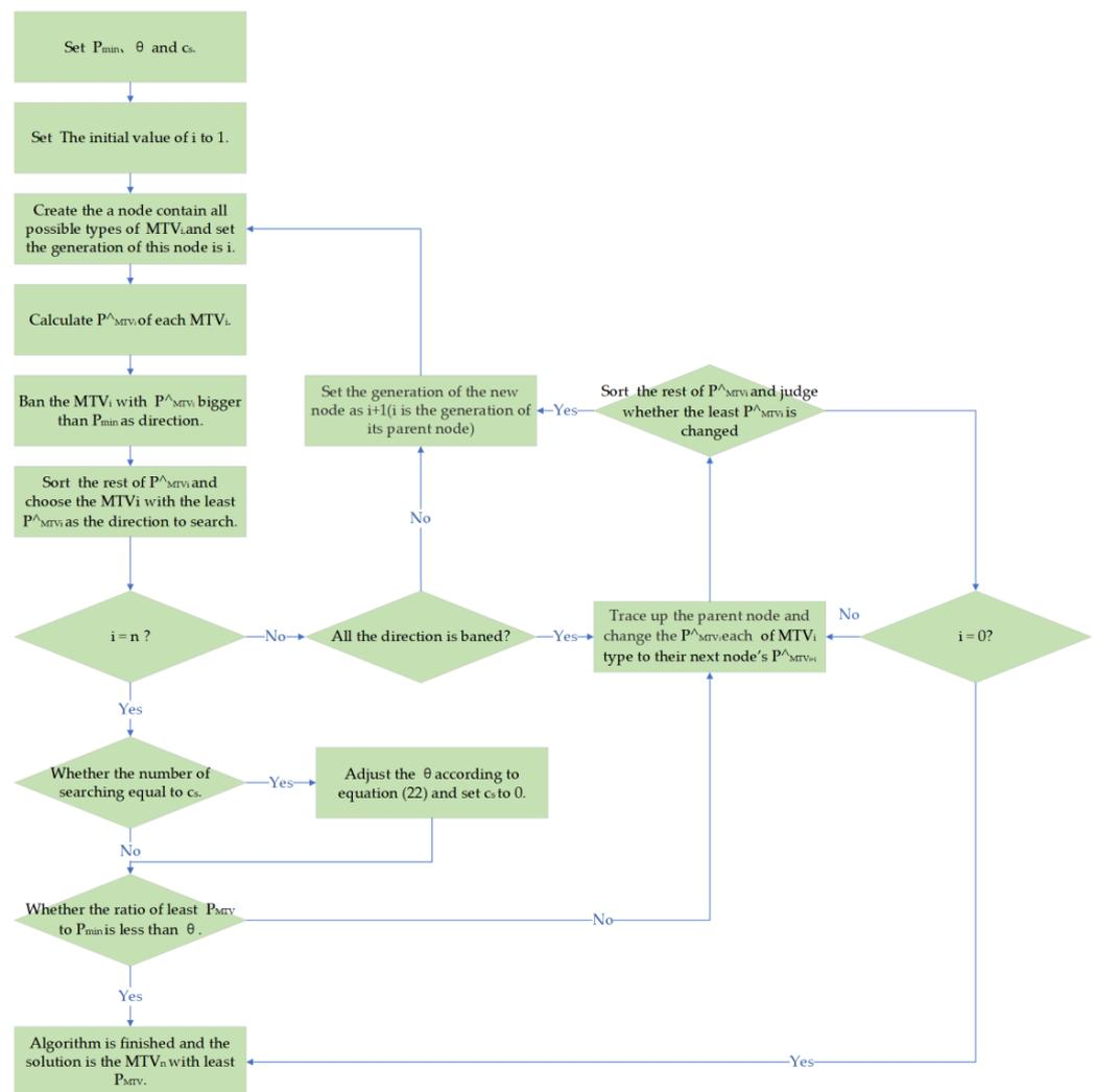
Figure 6. The flow diagram of heuristic search using the improved AO\*.
