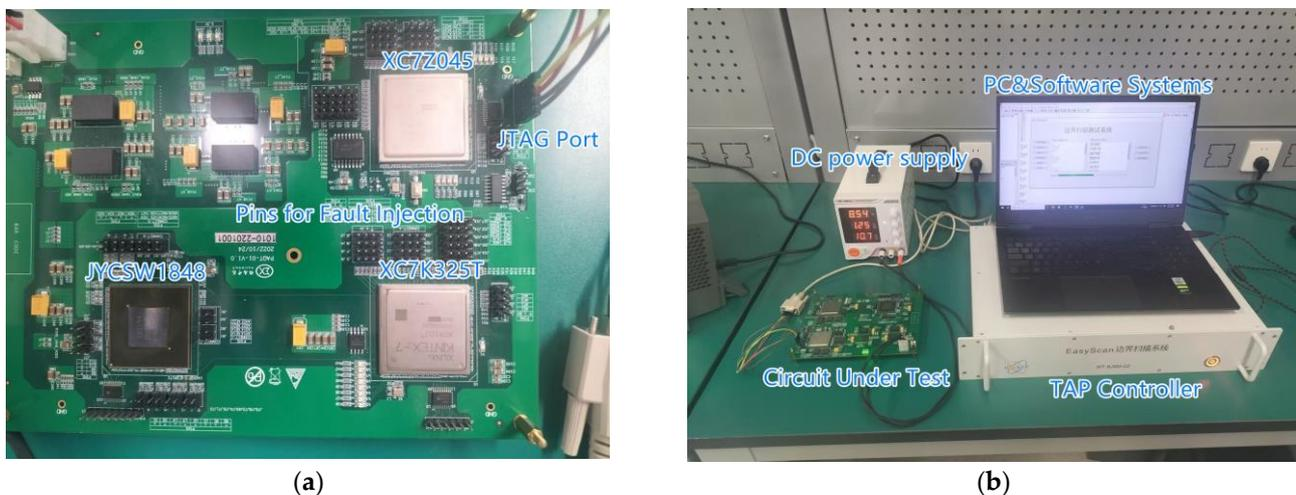
Figure 7. (a) The module under test; (b) Boundary scan test system.
