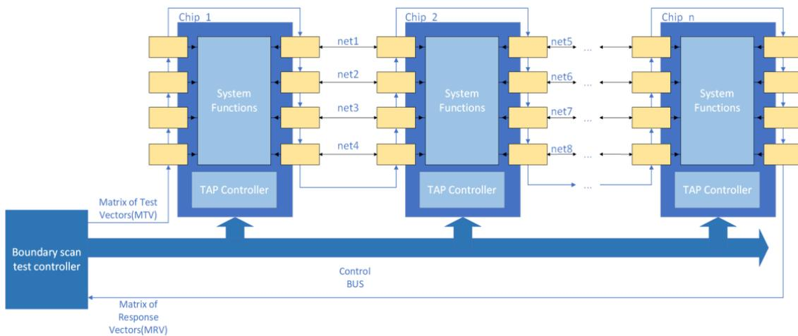
Figure 3. The structure of the boundary scan test.
