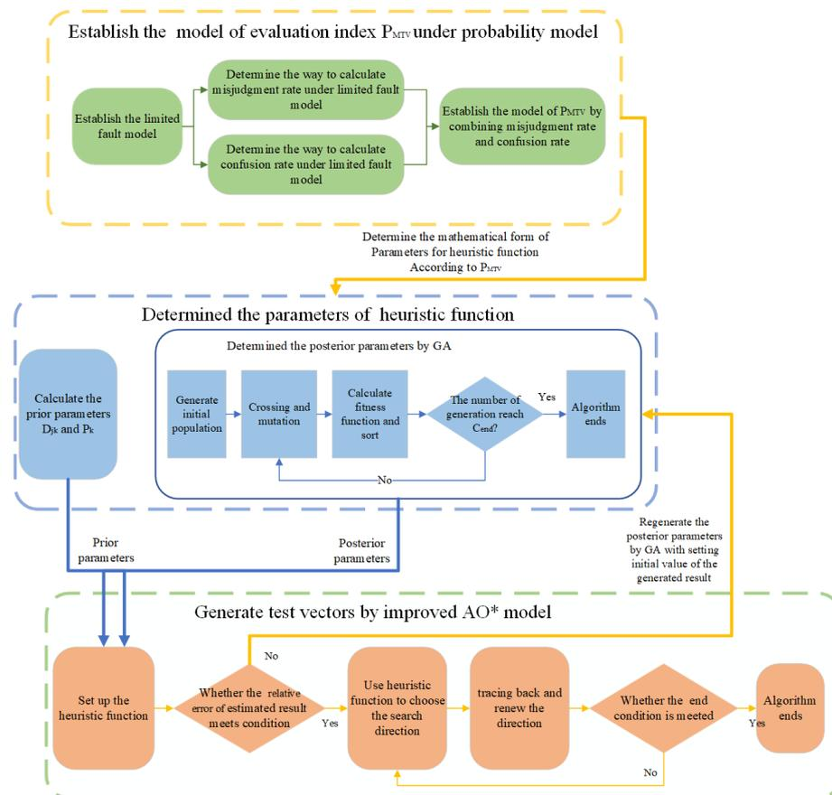
Figure 2. The process to establish the heuristic function and generate the MTV.
