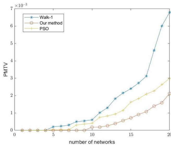
Figure 9. The  $P_{MTV}$  of MTVs generated by the three algorithms with the change in number of networks.
