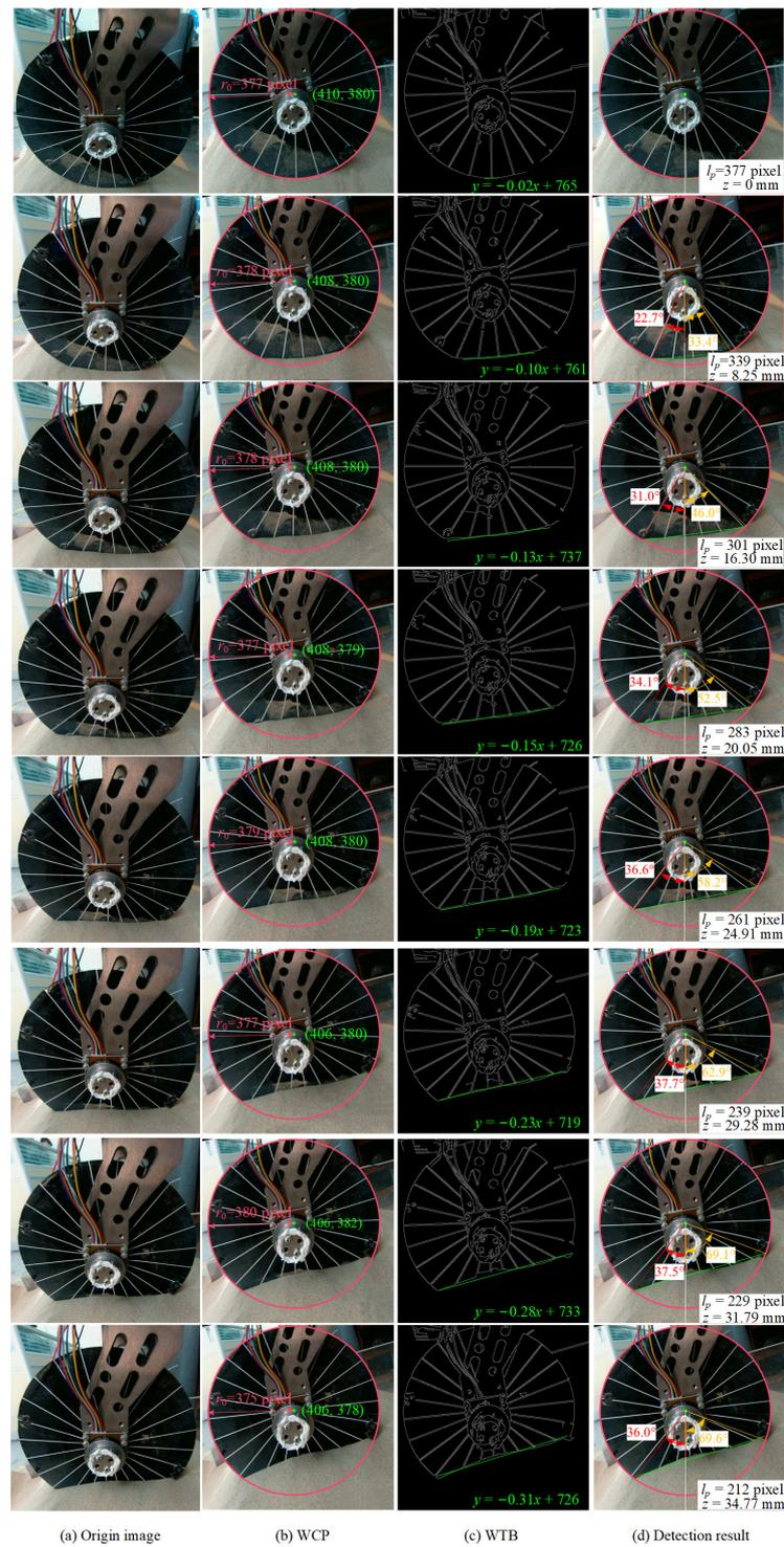
**Figure 7.** Results of eight different wheel sinkage depth tests: (a) Origin image; (b) WCP results; (c) WTB results; (d) detection results.
