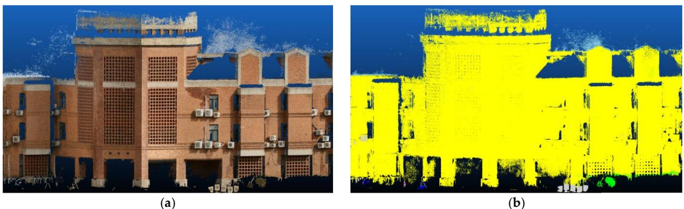
**Figure 10.** Dense point cloud reconstruction results: (a) the dense point cloud of the Tsinghua Life Sciences Building reconstructed using the original SGM; and (b) the dense point cloud of the Life Sciences Building reconstructed using sSGM based on semantics. Yellow points represent buildings, green points represent vegetation, gray points represent static-other, dark blue points represent bicycles, and light blue points represent sky.
