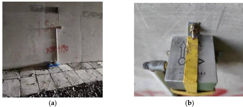
**Figure 10.** Site arrangement of measuring points. (a) Location of blasting vibrometer in tunnel, (b) The setting mode of sensor.
