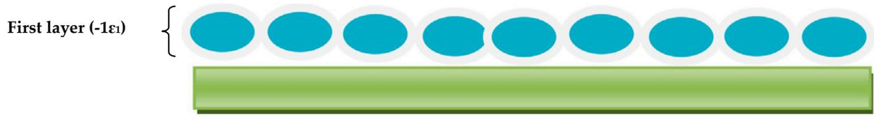
**Figure 2.** Schematic illustration of the distribution of the molecules adsorbed onto a solid according to the monolayer model with single energy.
