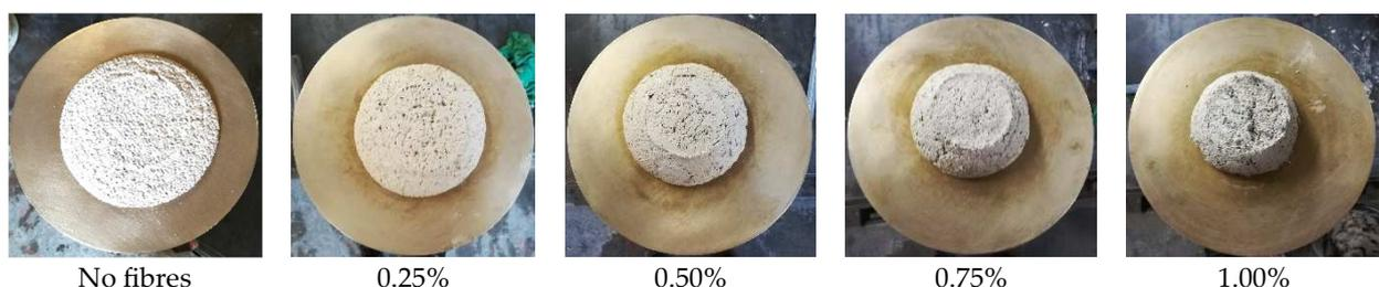
**Figure 6.** Flow table test results obtained for the different mixtures after 15 strokes.
