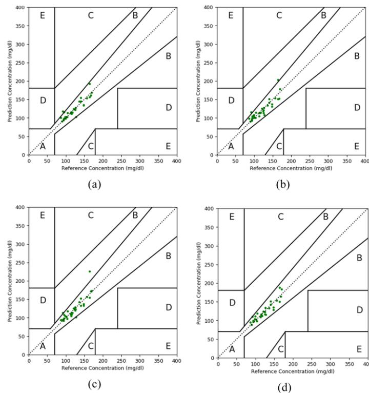
**Figure 9.** EGA plots for blood glucose estimation using PPG signals. (a) RF, (b) XGB, (c) LightGBM, (d) CatBoost.
