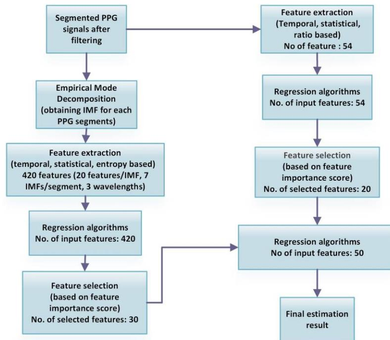
Figure 7. Flow chart of feature extraction and selection procedure.
