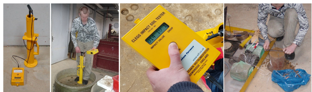
Figure 1. Device CIST-Type 31820 and homomorphic clay pavement subgrade models.
