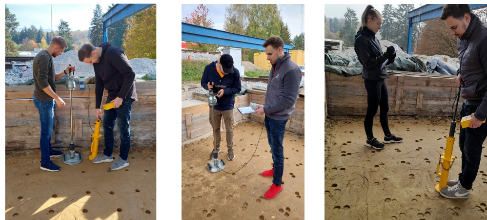
Figure 11. Measurements of clay subgrade on 17 October 2022 (left), 21 October 2022 (middle) and 3 November 2022 (right) by Clegg and LDD 100.
