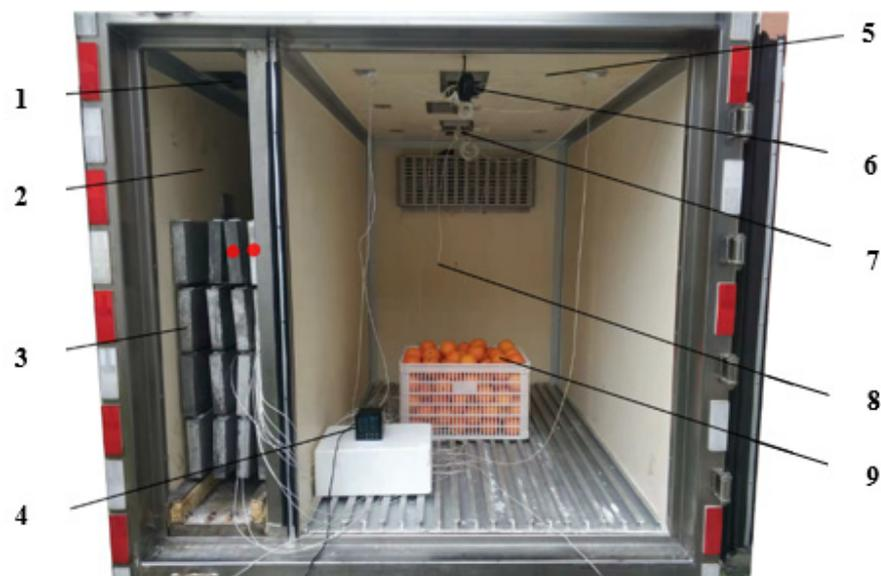
**Figure 2.** Temperature-controlled container with a cold energy storage system: 1—circulating duct; 2—cold storage area; 3—cold storage plate; 4—paperless recorder; 5—fresh-keeping area; 6—fan (outlet); 7—fan (inlet); 8—PT100; 9—navel oranges.
