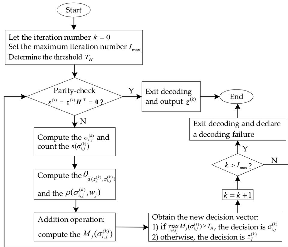
Figure 3. The flow diagram of the MRAI-LDPC decoding algorithm.
