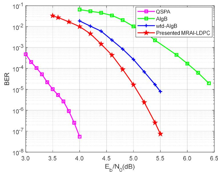
**Figure 6.** The decoding performance of the  $F_{16}(255, 175)$  QC-LDPC code.
