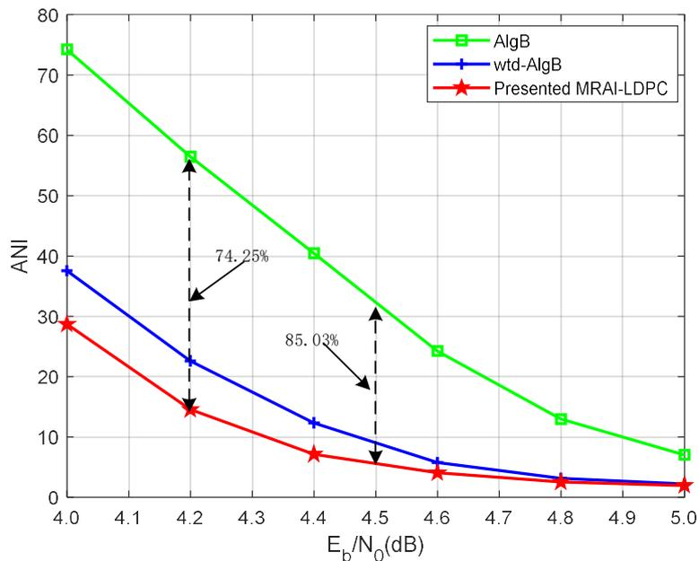
Figure 5. The average number of iterations under the  $F_{16}(225, 147)$  QC-LDPC code.
