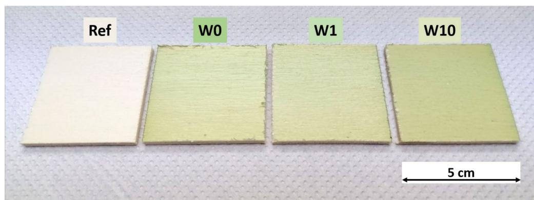
**Figure 4.** Appearance of the coatings containing spirulina-based pigment and carnauba wax filler [41]. Modified from *Progress in Organic Coatings*, 182, M. Calovi, S. Rossi, Synergistic contribution of bio-based additives in wood paint: The combined effect of pigment deriving from spirulina and multifunctional filler based on carnauba wax, 107713, Copyright (2023), with permission from Elsevier.
