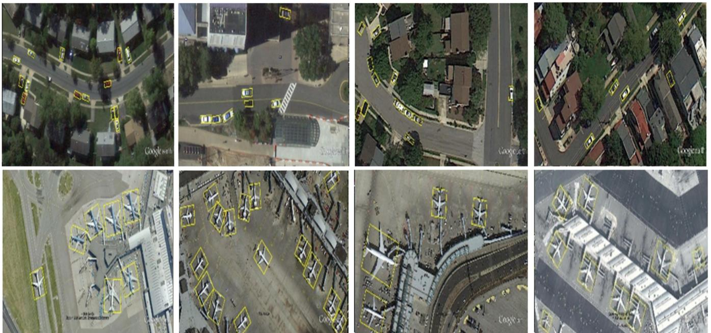
Figure 7. The detection effect of this method on the UCAS-AOD. The yellow box represents detection results.
