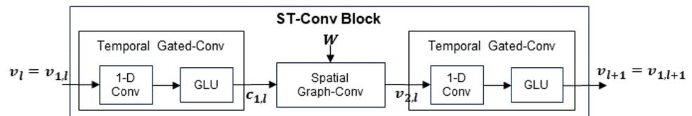
**Figure 2.** ST-Conv block pipeline.
