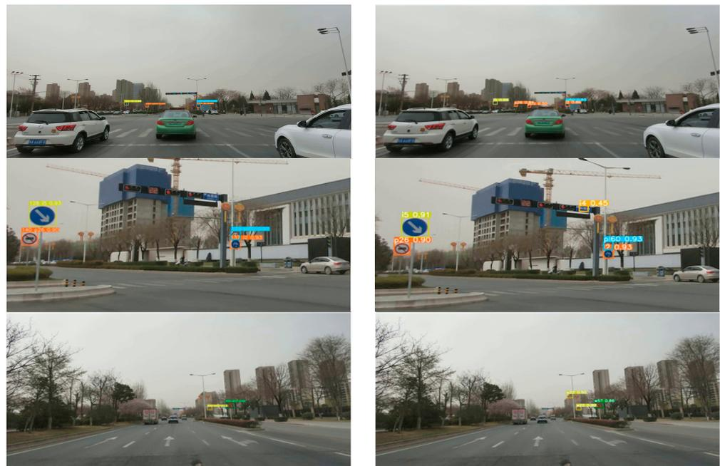
**Figure 10.** Comparison of images collected from real vehicles. The left column represents the results of the standard YOLOv5s network model image, and the outcomes of the enhanced network model suggested in this article are shown in the right column.
