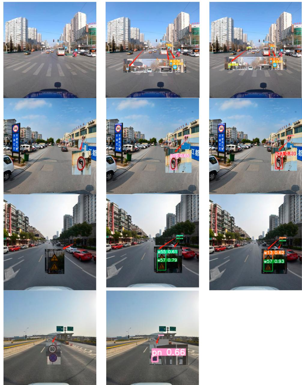
**Figure 9.** Comparison of actual road scene. The results of detecting images using weights derived from the standard YOLOv5s network model trained on the augmented dataset are displayed in the middle column, undetected images of actual road scenes are displayed in the left column, and the results of detecting images using weights derived from the improved network model proposed in this paper trained on the augmented dataset are displayed in the right column.
